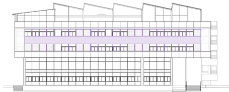
Figure 132. Grid support system to allow architectural researchers to incorporate their own prototypes on the face of the building.
