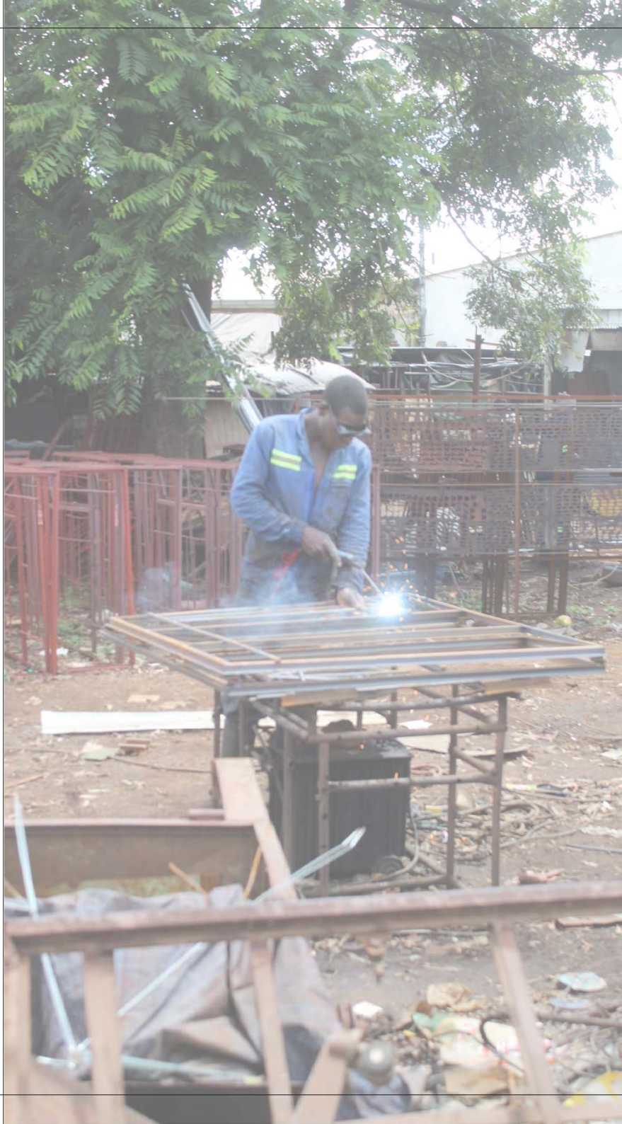
1_16. Tradesman welding steel window frames at Magaba.
