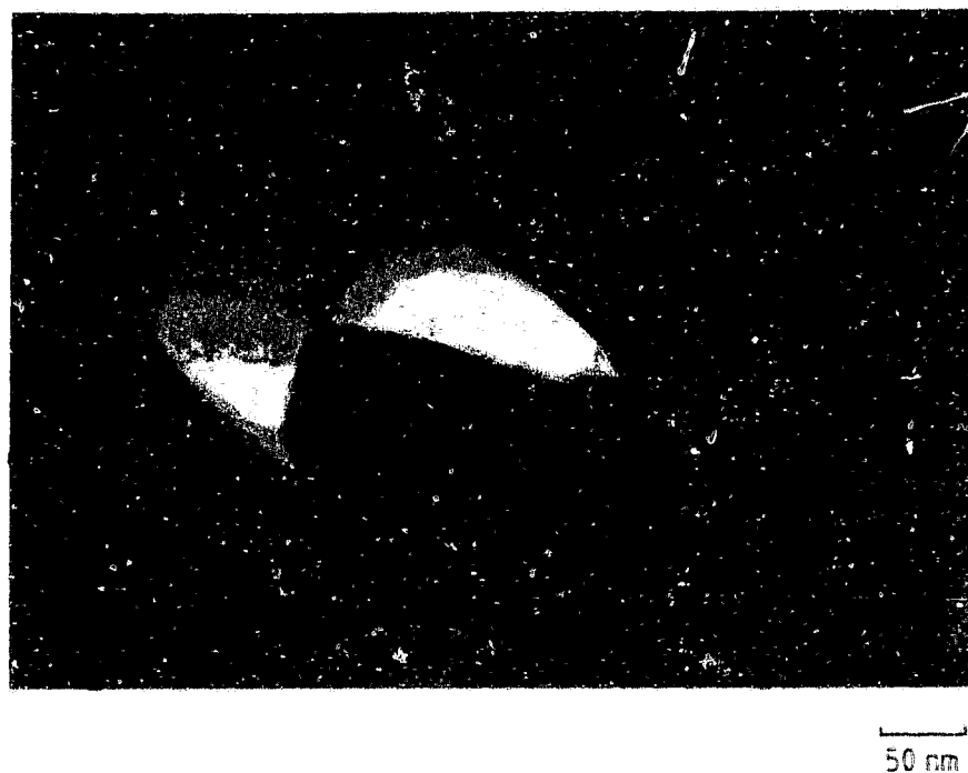
Figure 2.33 BF micrograph showing the plate-like morphology of a \eta particle
