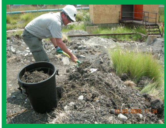
Figure 3.2: Photograph demonstrating how RBMR waste soil samples were collected.
