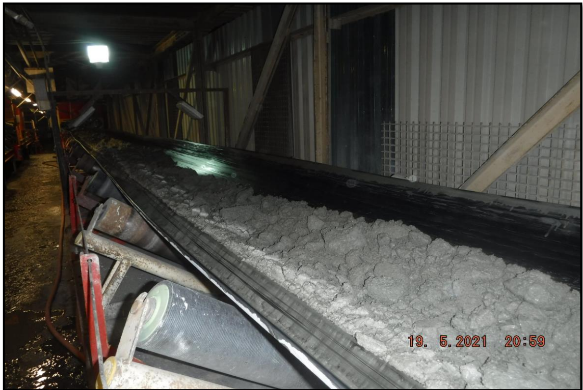
Figure 5-16: Surface belt audit to check fragmentation (Nair, 2021)
