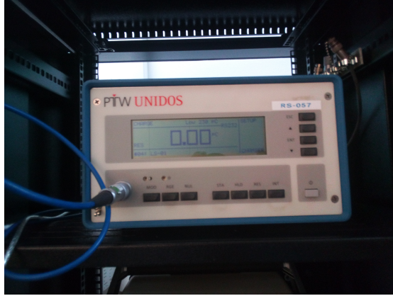
Figure 8: PTW eletrometer used for standard dosimeter calibrations at the NMISA.
