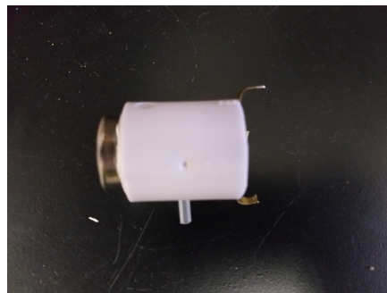
Figure 34: Discharge tube with porous electrodes (side view).
