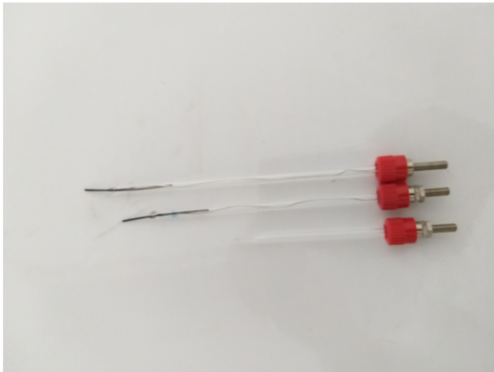
Figure 19: Glass-insulated probes in various sizes.
