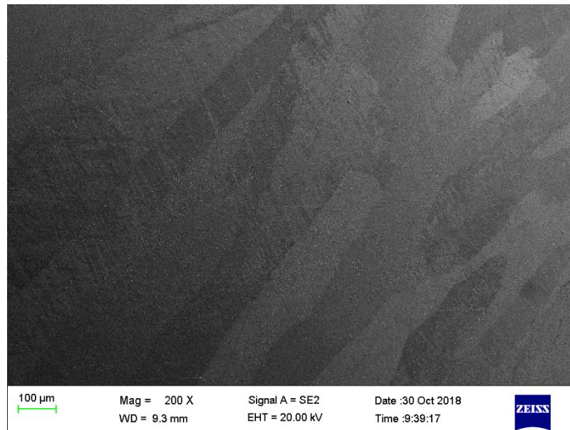
Figure 4.76. SEM-SE image of \text{Co}_6\text{Fe}_{44}\text{Pd}_{50} (at.%), Alloy 2 annealed at 650^\circ\text{C} for 1000 h showing light and dark grains.
