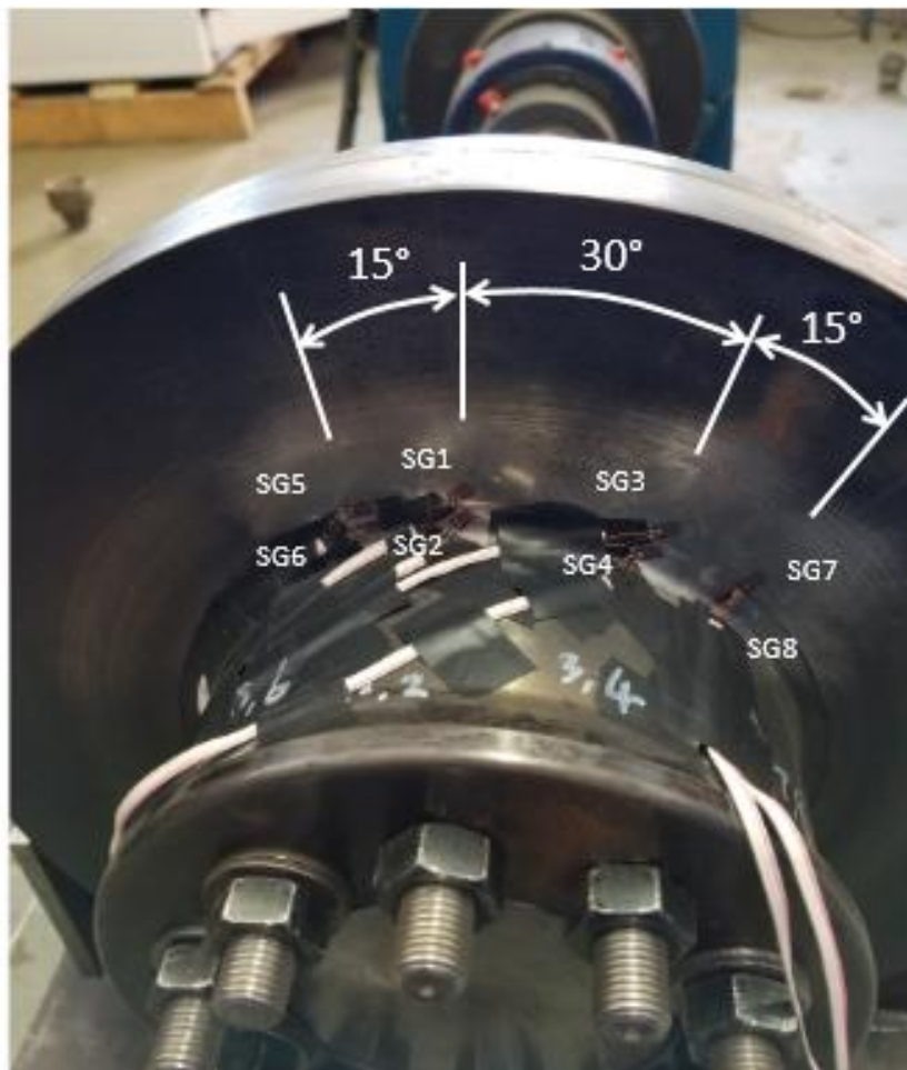
Figure 21: Eight uniaxial strain gauges installed for applied torque load test (SG: strain gauge)
