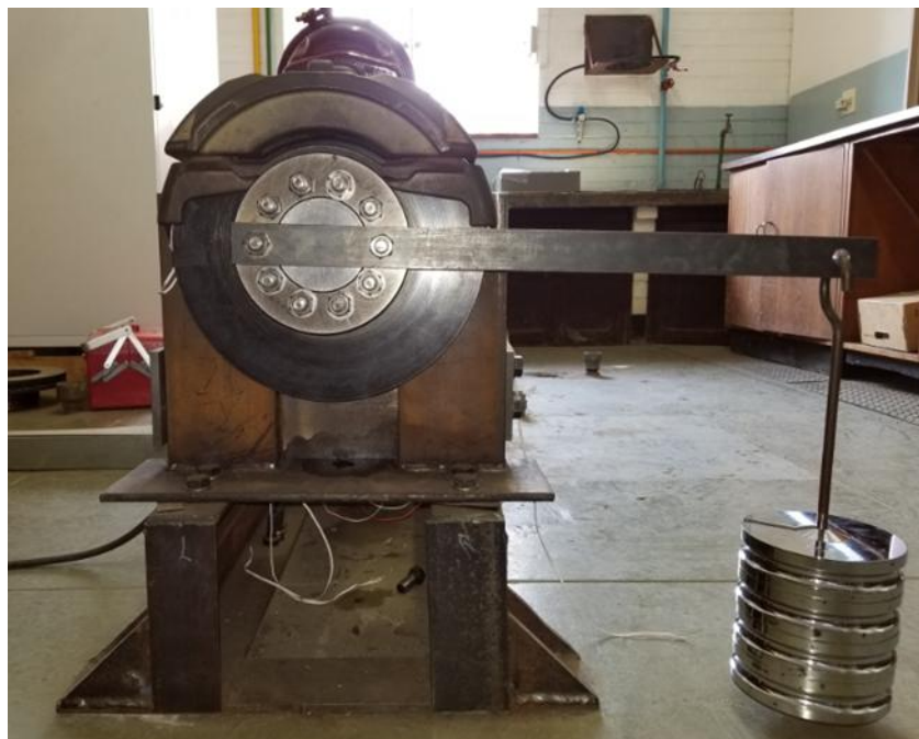
Figure 27: Mass hanger with calibration weights applying torque to the shaft through a flat bar
