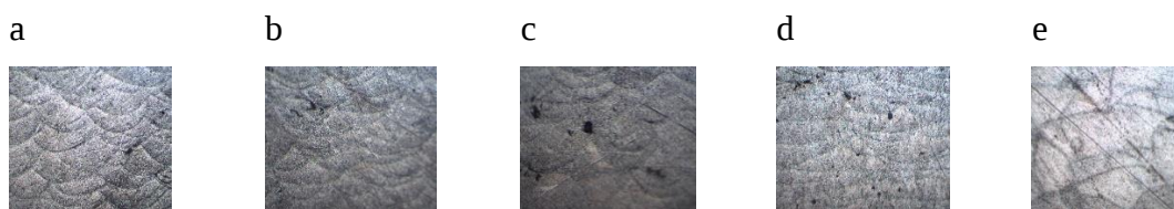
Figure 56: Optical microscopy of cross section of as built samples near the middle (a) 1.2 mm, (b) 2.6 mm, (c) 5.6 mm, (d) 9.6 mm and (e) 13.6 mm
