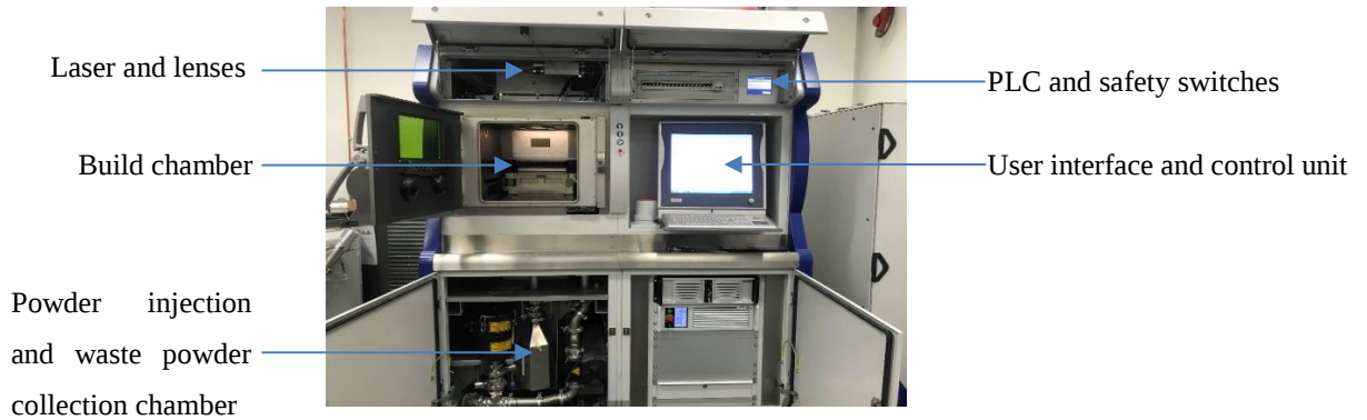
Figure 30: SLM 280 machine with compartments open [70]
