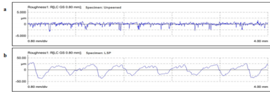
Figure 12: Surface roughness profile for (a) as-built and (b) peened samples [53].
