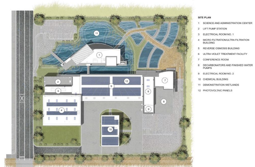
Figure 4.5.1: Advanced Water Purification Facility Site Plan
