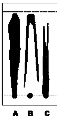
Figure AIII-8 A diagrammatic representation of TLC patterns observed in microperoxidase samples that were purified using the Amicon® cell. The patterns were independent of concentration and were grouped according to tailing ( A ) which was typically observed when the spotting solution was used immediately after preparation, eclipsing ( B ) which was typically observed when the spotting solution had been allowed to stir for ca. 2 hours or feathering ( C ) which was observed when the spotting solution had been allowed to stir for ca. 4 hours.
