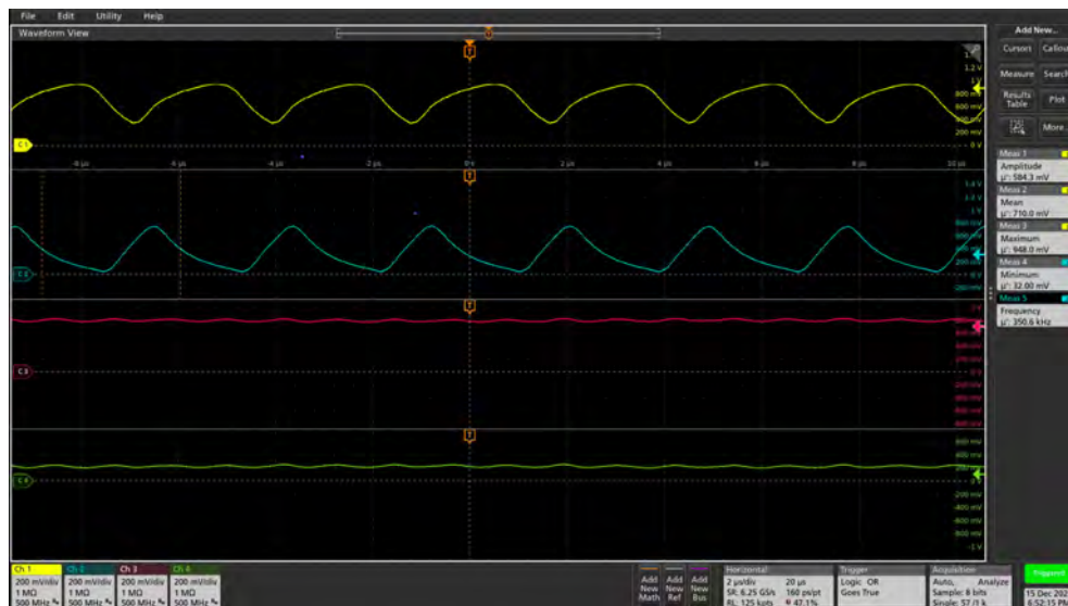
Figure 7.12: Instability with Isolation amplifier.
