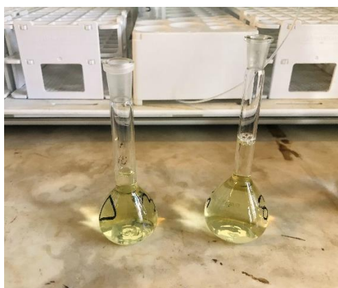
Figure 22: Diluted standard solutions (25 mL) of SS/ISSA prior to AAS analysis
