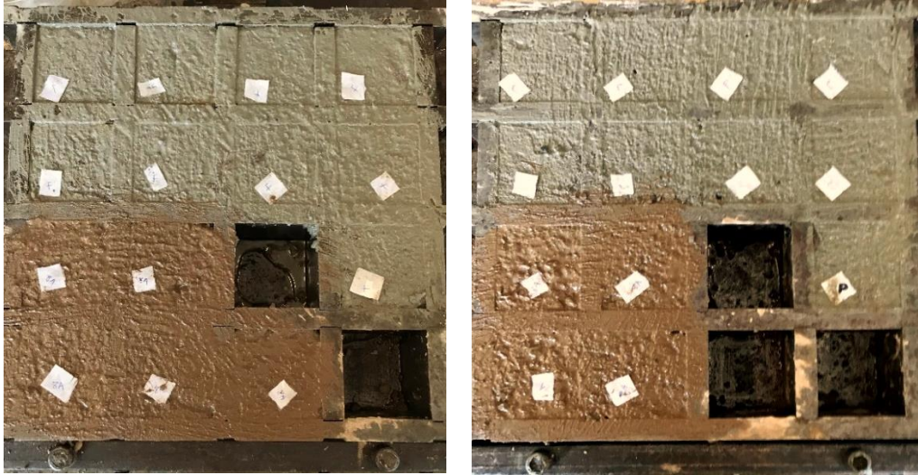
Figure 28: Cube moulds filled with cement mortar
