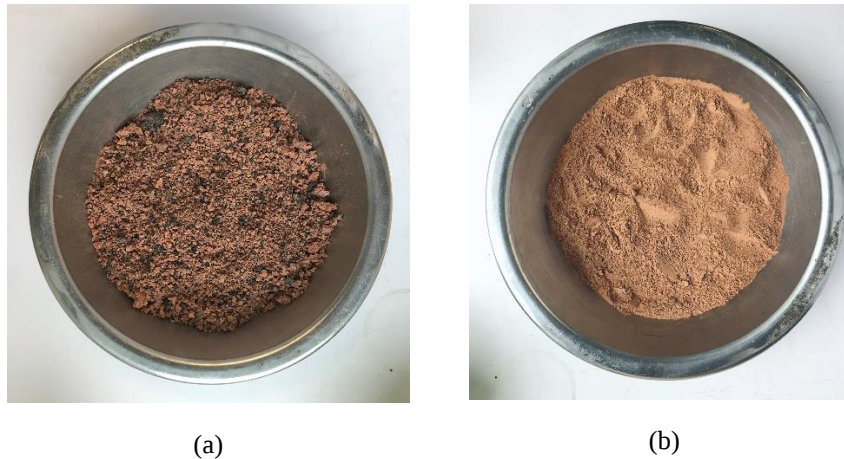
Figure 20: Incinerated sewage sludge ash (a) and pulverized incinerated sewage sludge ash (b)
