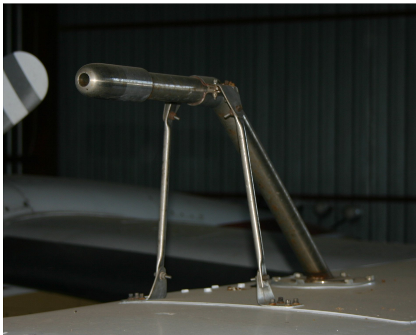
Figure 2.5: A close-up of the inlet nozzle on the Aerocommander ZS-JRA.
