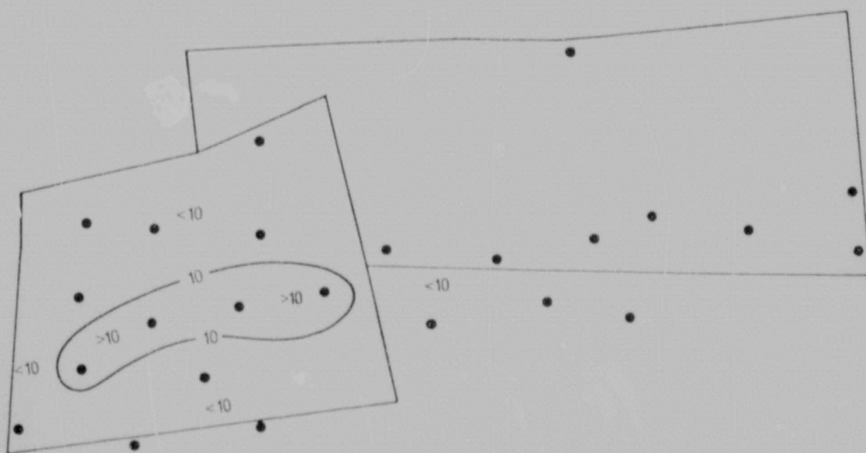
Figure 17 : A percentage map showing the estimated variation in total chert content within the Lower Dark Dolomite Zone. Contour values in per cent.
