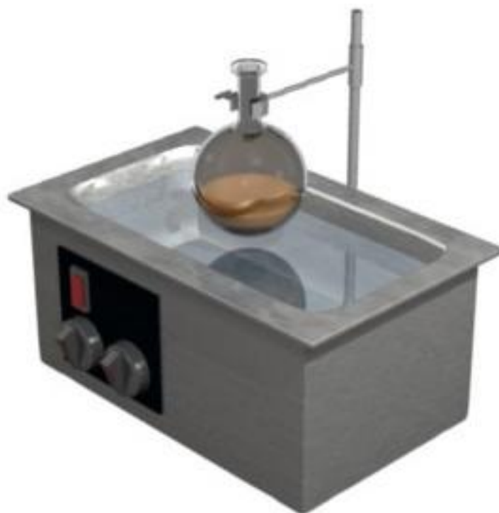
Figure 8: Sonochemical Reaction Set-Up Including Ultrasonic Cleaning Bath
