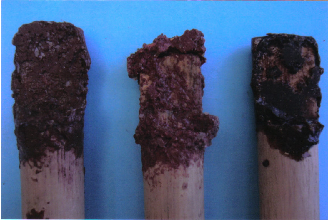
Figure 6.3 The adhesives left on the hafts of Tools 51, 21 and 68. Tool 51 was successful, but broke months afterwards, whereas Tools 21 and 68 broke during the activities. The bubbles, and inconsistent and crumbly nature of the adhesives, especially those on Tools 21 and 68, are clearly visible.
