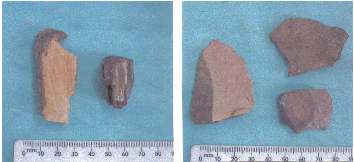
Figure 3.4.7 Two examples of the colour changes that occur when ochre is heated. The unheated pieces are those on the left side of each picture. The heated pieces are darker, but sometimes only slightly.
