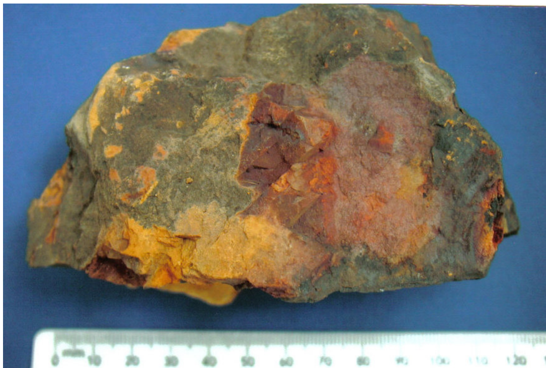
Figure 3.3.3 Snuff-box shale piece showing ‘pockets’ of soft yellow and red colouring.
