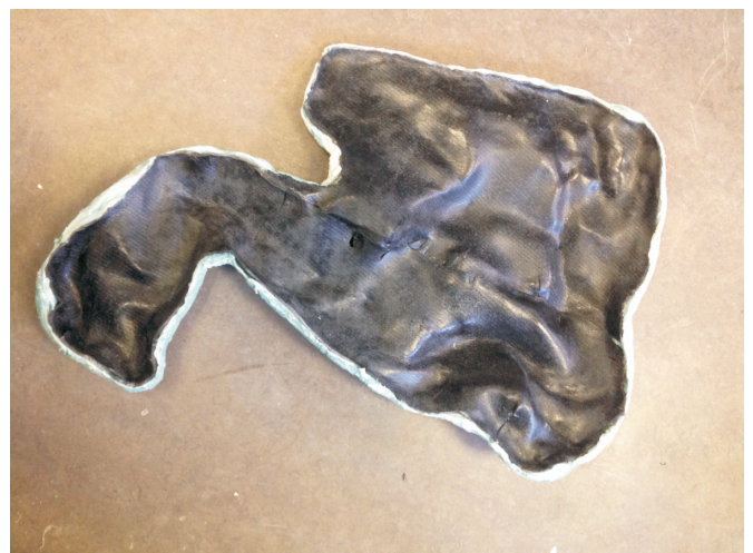
Figure 7. Plastecine removed from the hardened resin jacket and plastazote foam layer glued into place.
