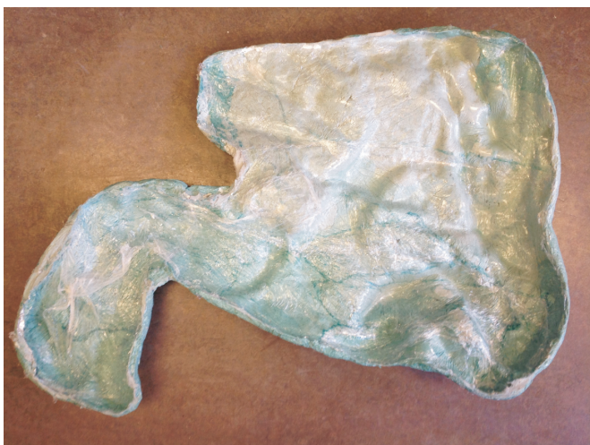
Figure 6. Resin being applied over the cling film covered plastecine, to be followed by a second cling film layer added over the entire surface.
