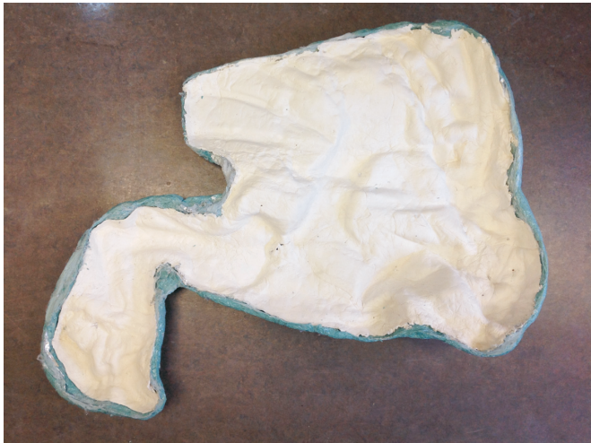
Figure 4. Application of a rolled, removable plastecine layer creates space within the jacket for the addition of a Plastazote® foam lining.
