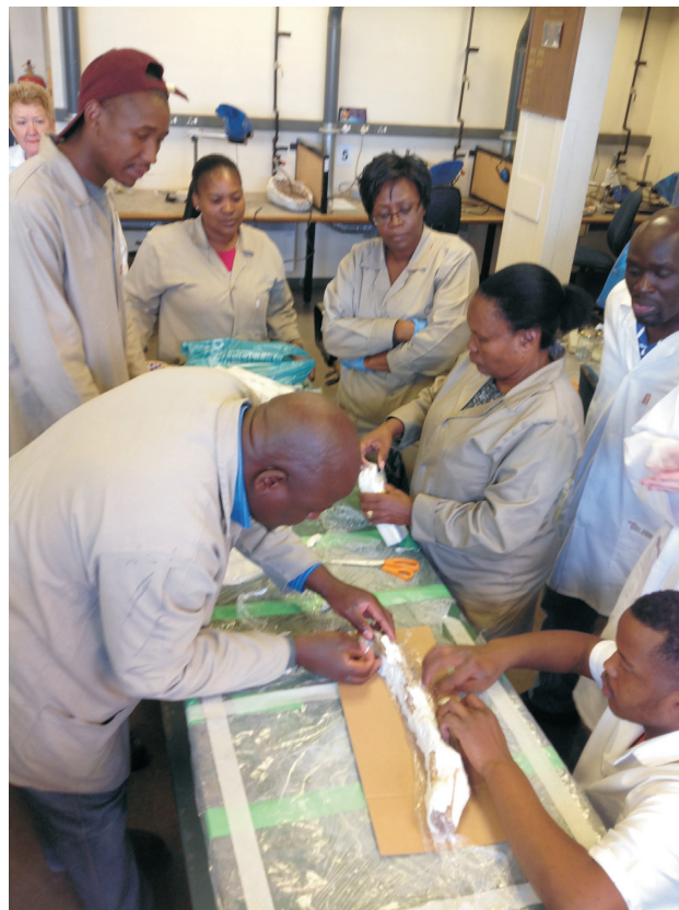
Figure 2. Checking for, and filling, undercuts and voids with plasticine.
