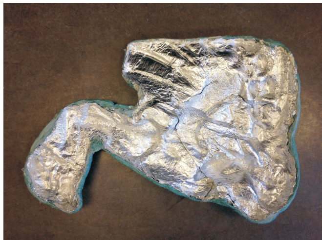
Figure 3. Blocks 5 and 6 protected by aluminium foil and cling film.
