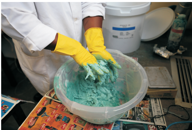
Figure 5. Resin being mixed with the activator. Note the need for personal protective equipment.
