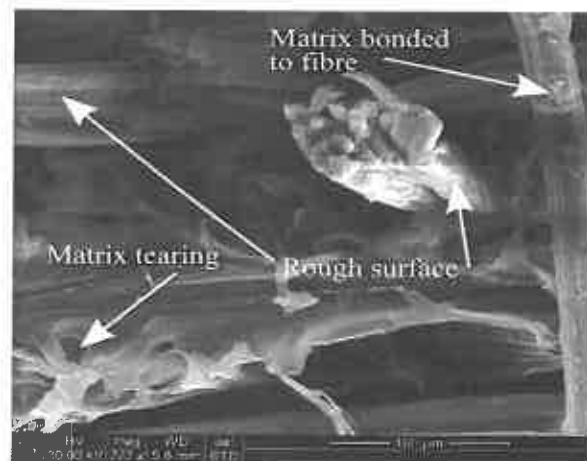
Figure 5.14: NaOH - PP Matrix - zoomed in section of tensile specimen
