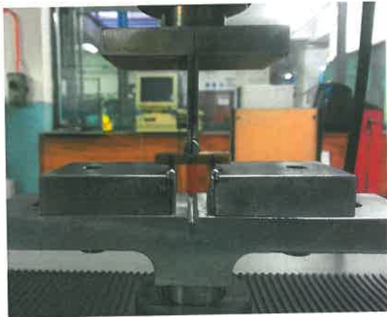
Figure 4.21: Short Beam Shear Rig
