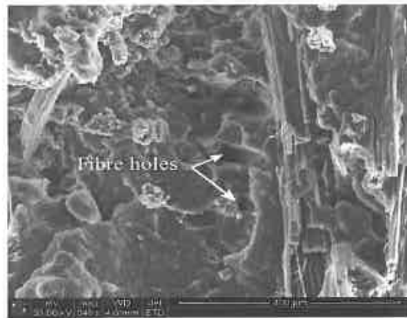
Figure 5.38: SEM images of impact specimens using 5% MPS treated fibres with clay matrix
