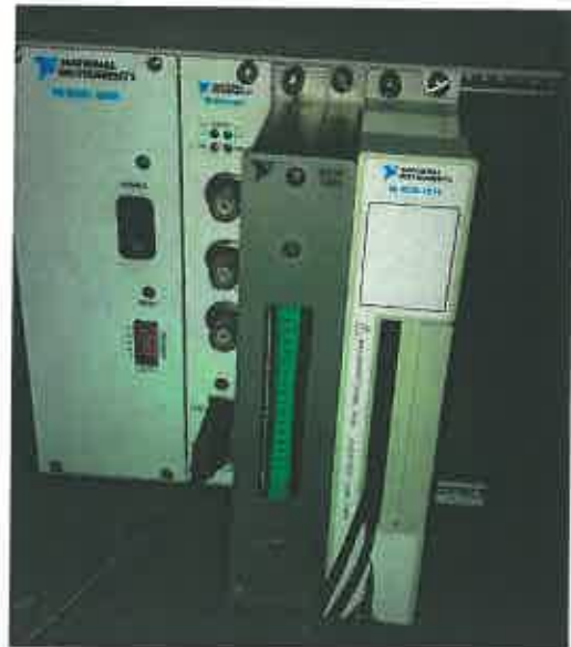
(b) DAQ used to collect force and deflection data
