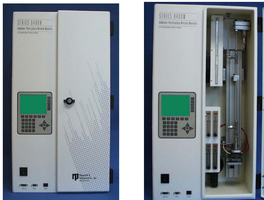
Figure 6. Photograph of the Ambient Particulate Nitrate Monitor's pulse generator outside view (left) and inside view (right).
