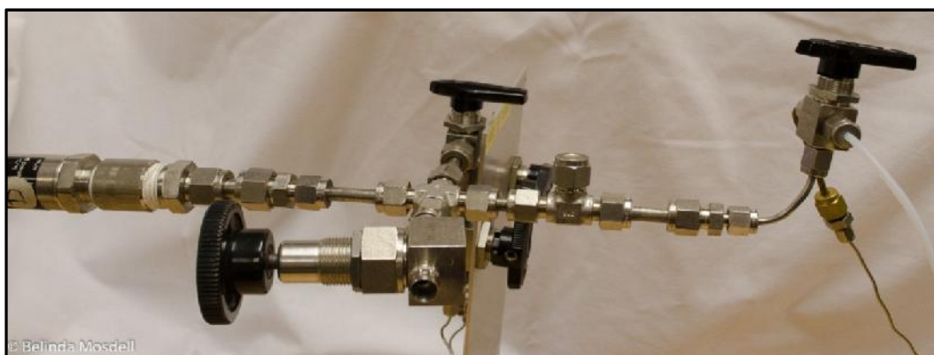
Figure 33: Sample holder for \text{CaC}_2/\text{H}_2\text{O} reaction
