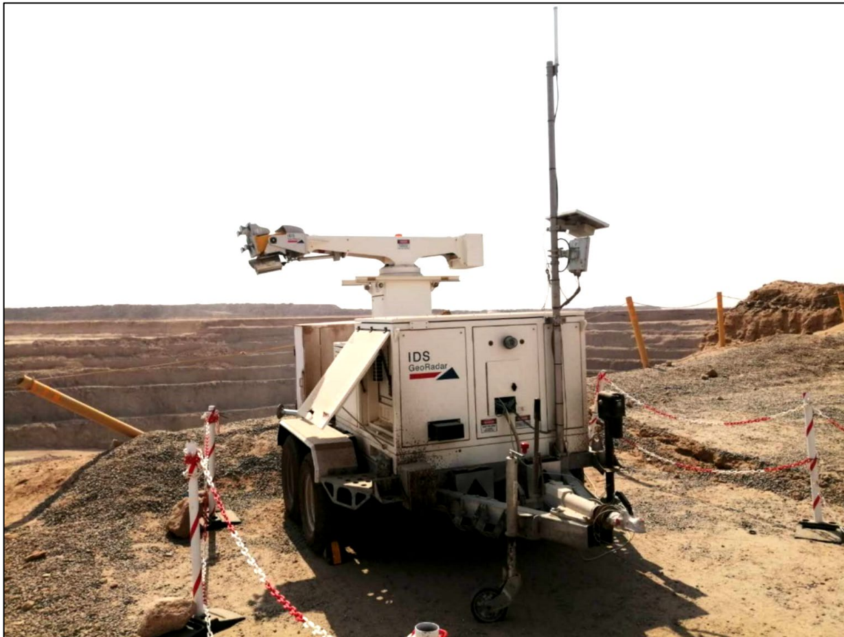
Figure 2-11: IBIS-ArcSAR radar deployed in an open pit operation, photograph taken at Husab mine (Namibia)
