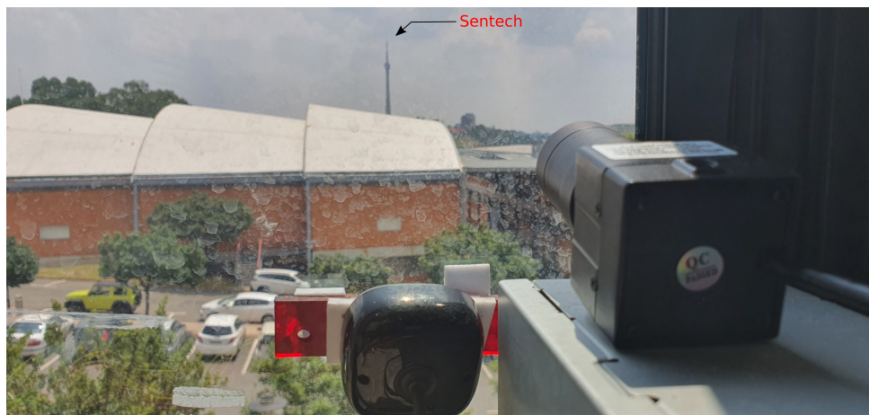
Figure 3.7: Image of the slow speed cameras and the view they film. The camera on the left is a webcam with a maximum record speed of 30fps. The camera on the right has a maximum record speed of 100fps.
