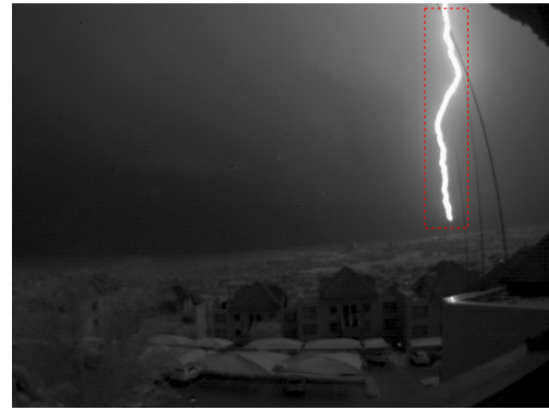
(d) Frame showing the first subsequent return stroke (red) for the upward lightning event.
