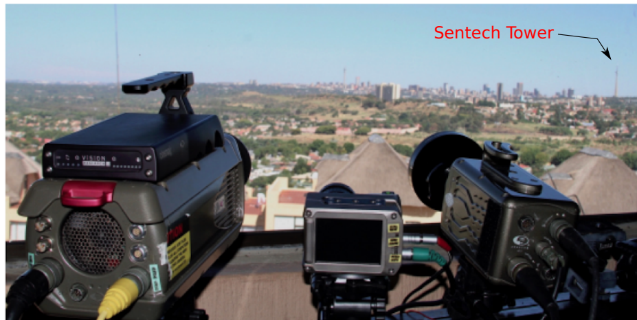
Figure 3.6: Photograph showing the high speed cameras and the view that is recorded. The camera on the left is the Phantom v310 while the camera on the right is the Phantom v7.
