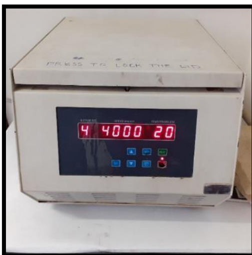
Figure S5: Centrifuge machine used for the second trial with the settings displayed.
