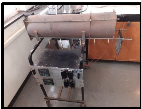
Figure 5.2: CVD reactor system used to dope the OLCNs with ammonia gas.
