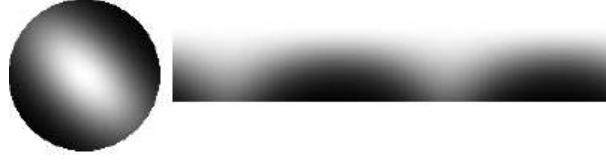
FIGURE 2.7: The Gaussian weight distribution provides more weighting to foreground regions that are likely to contain people and less weight to the background regions of the image [5].
