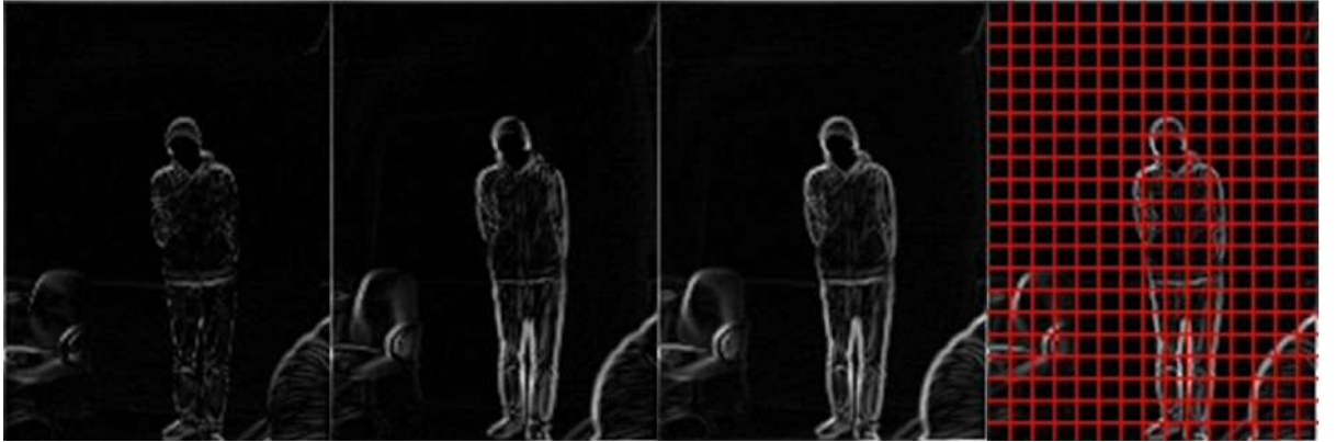
FIGURE 4.3: The horizontal gradient I_x (1st), vertical gradient I_y (2nd), magnitude of gradients M (3rd) and the cell division of the magnitude of gradients image (4th).
