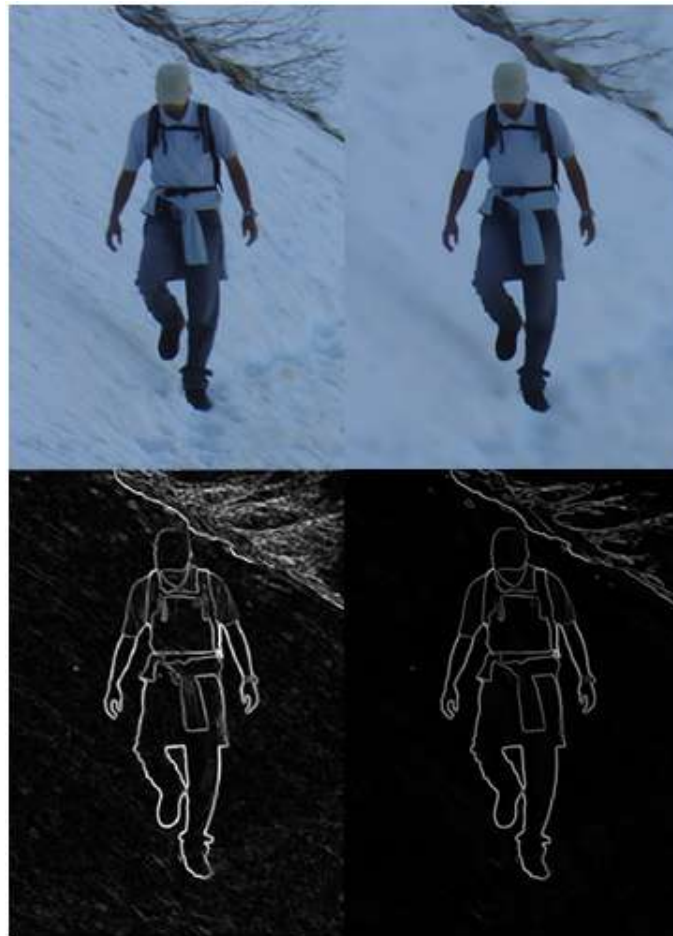
FIGURE 7.1: Cartooned image, colour unification for better boundary edge extraction. Top left is the original image. Followed by its cartooned version (top-right). The corresponding magnitudes of gradients images are shown below it [1].
