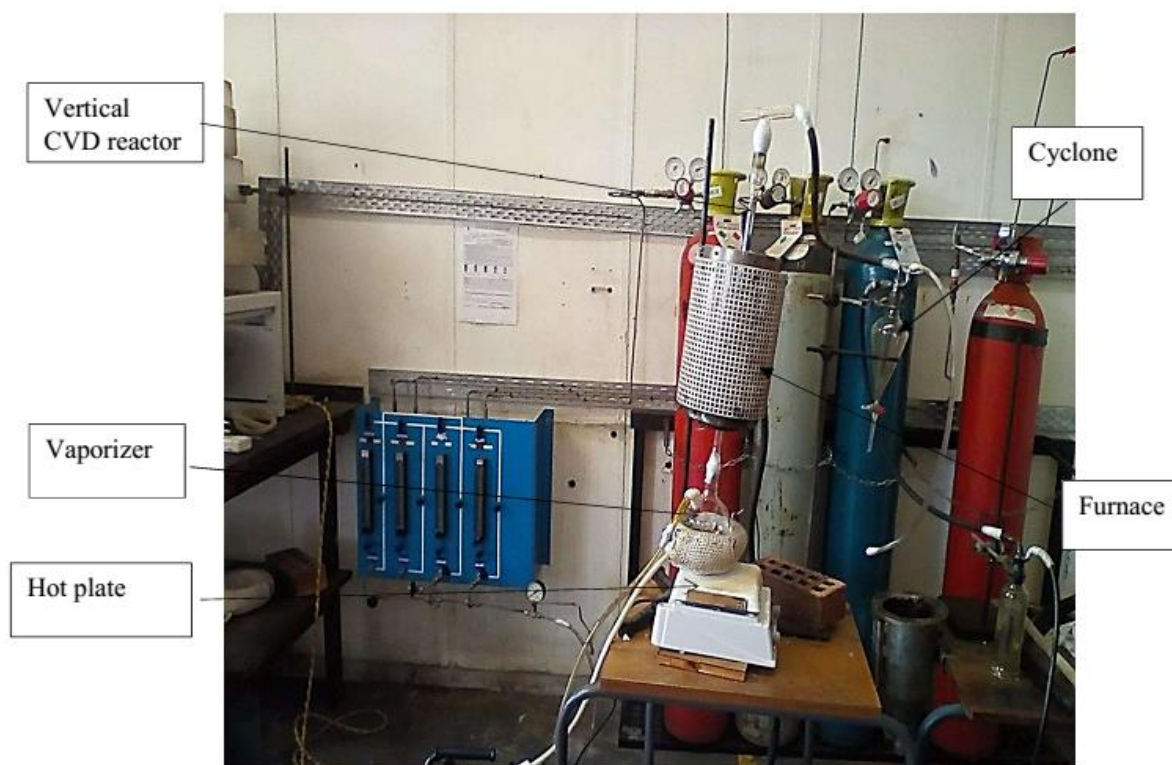
Figure 1: An experimental set-up for CNT production.
