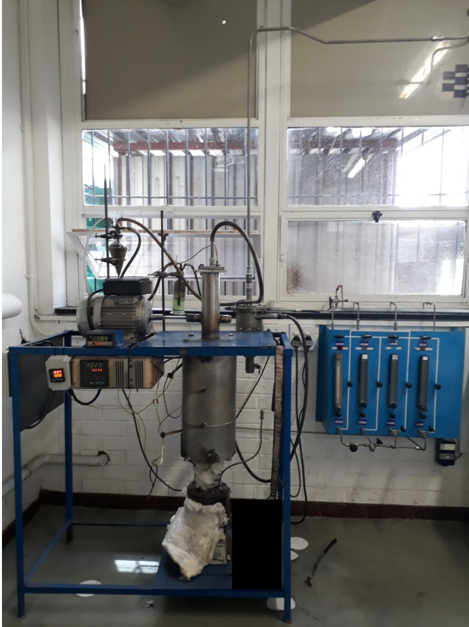
Figure A1: Floating catalyst chemical vapour deposition reactor with direct spinning set-up in operation
