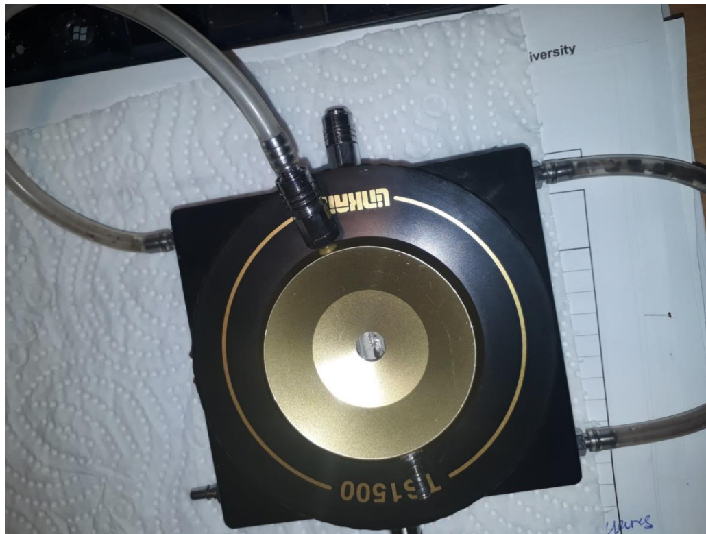
Figure 3.2 Photograph of the micro-Raman containing CNT yarn placed on alumina substrate and held on with silver paste
