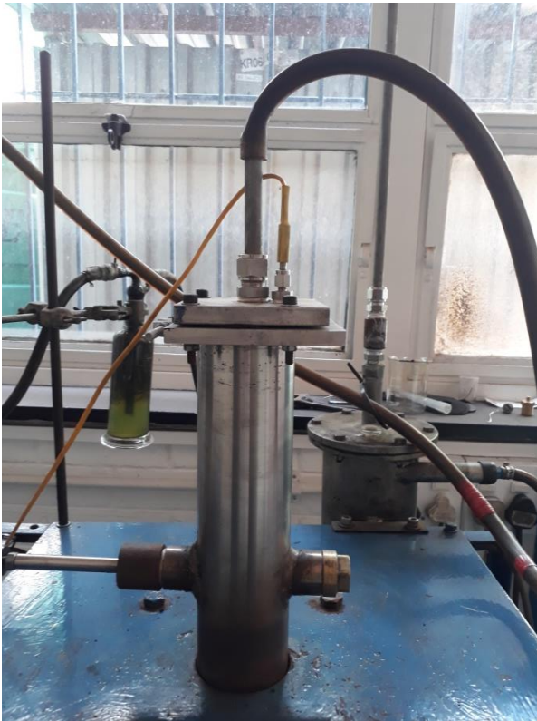
Figure A6: Upper part of FCCVD reactor set up
