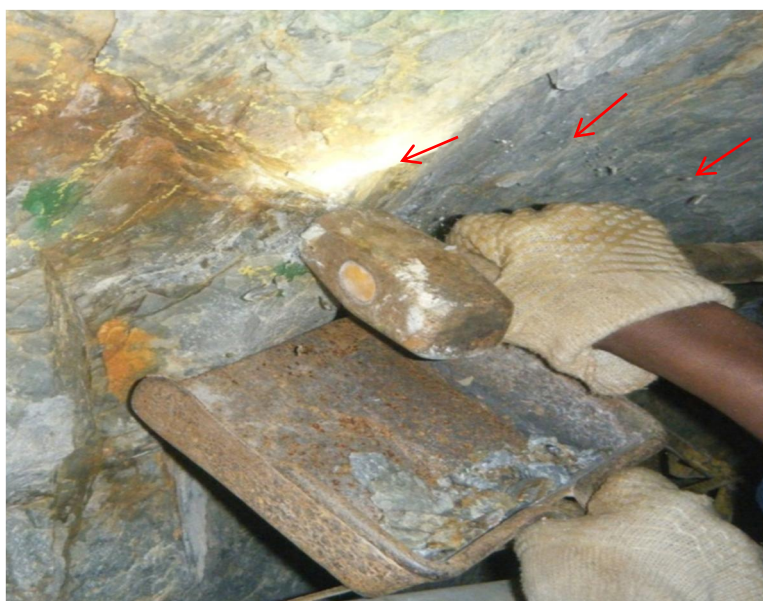
Figure 5.2: Sample loss clearly visible when the chipper are using use a hammer to collect sample
