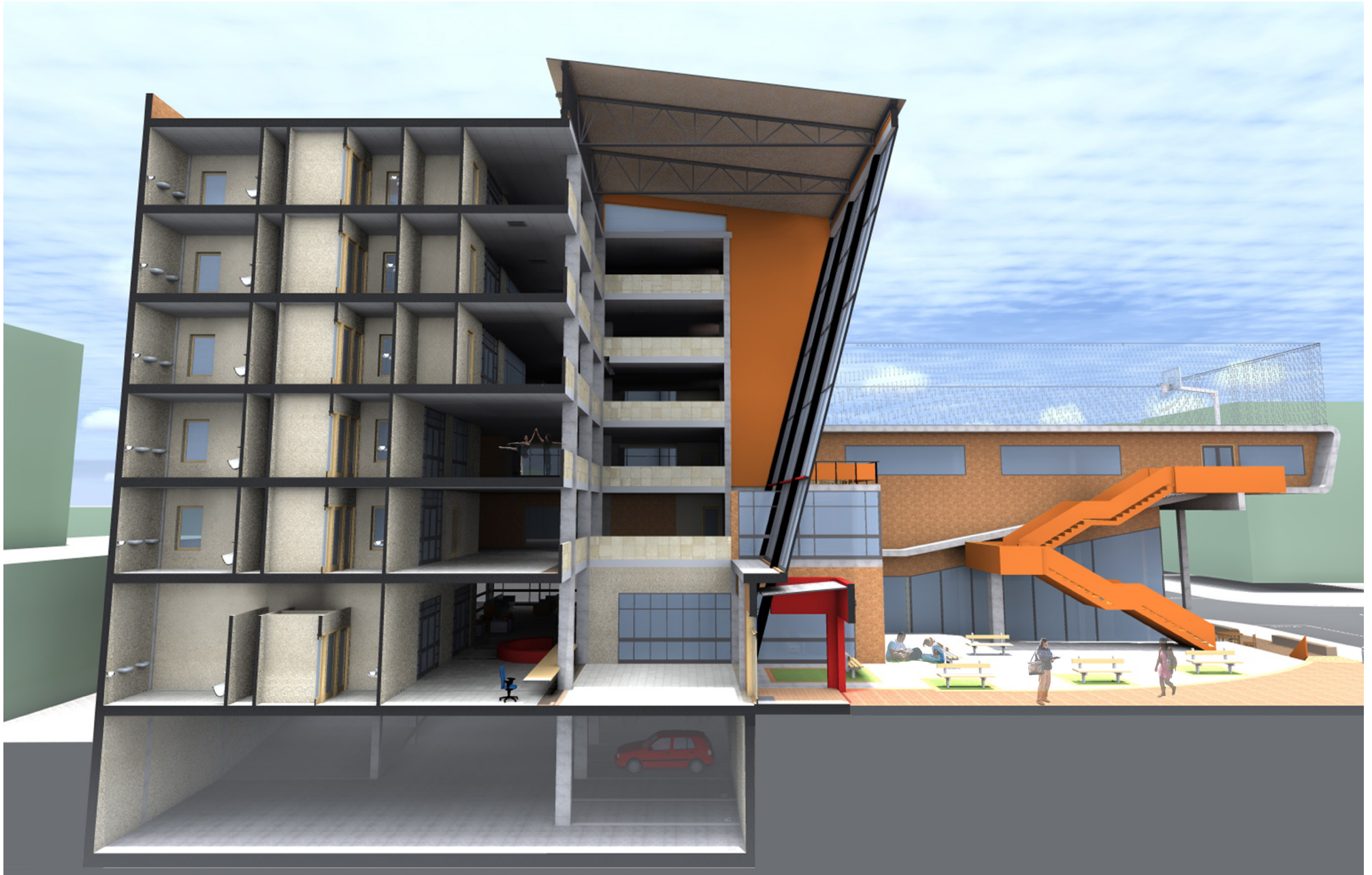
Cut-away section showing atrium and internal spaces
