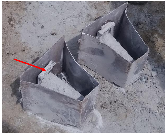
Figure 3-5 RC sub-sampling sample cups with cup handles (highlighted with the red arrow) that restricting the fall of sample
