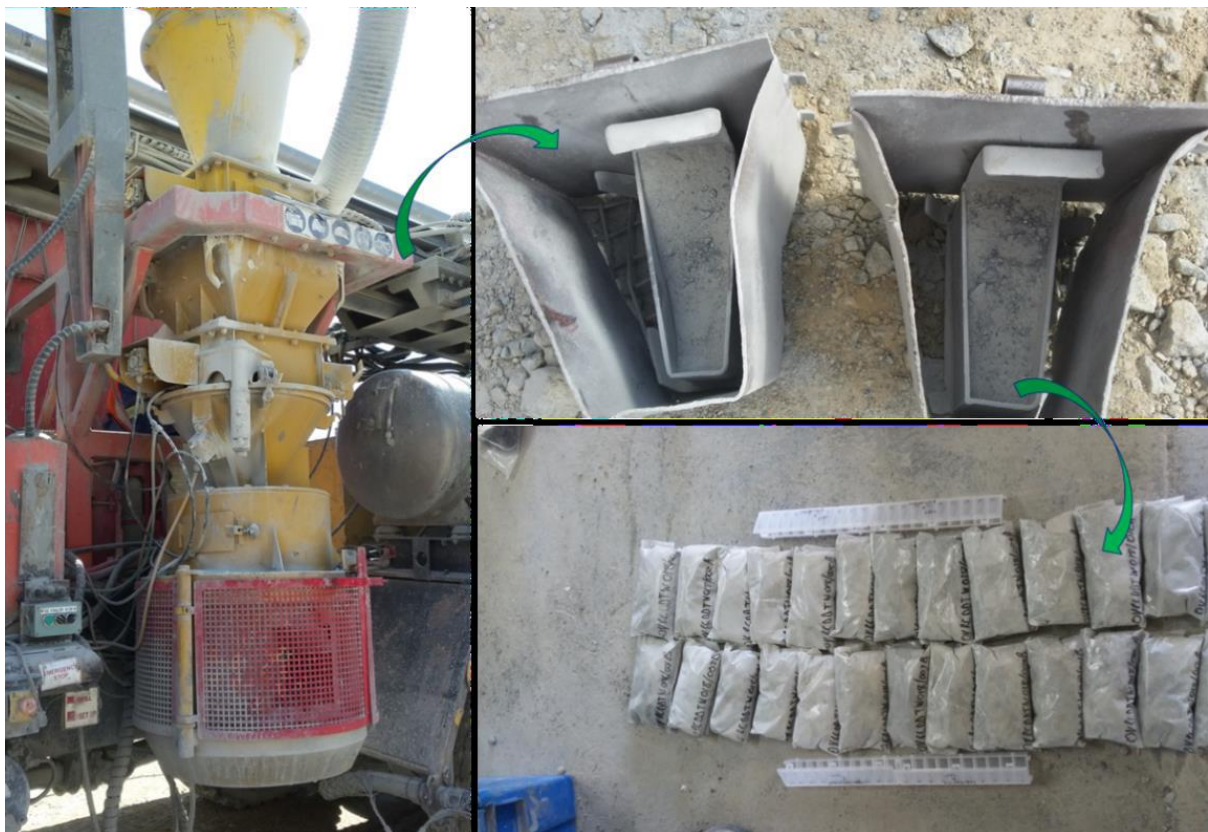
Figure 3-3 Reverse circulation drilling rota-port splitter, sample cups and samples used for grade control
