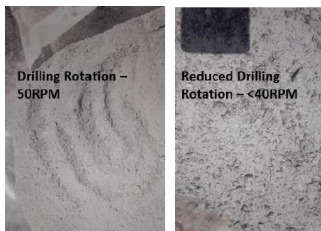
Figure 8-1 Effect of drilling rotation speed on sample fineness, demonstrating slower drilling speed produce sample chips with coarser factions
