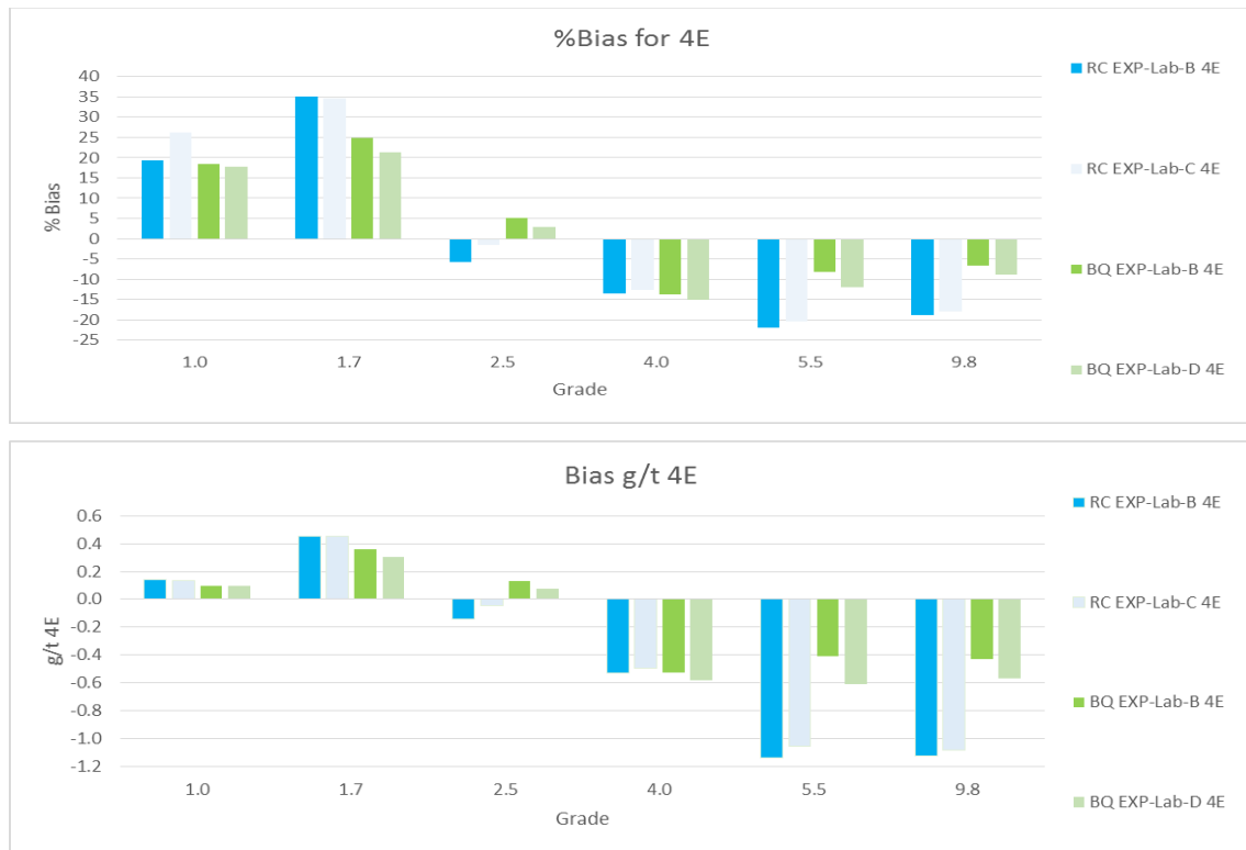
Figure 7-9 Systematic errors RC vs. BQ sampling at quantified at the GCDPs, in g/t 4E and %Diff 4E
