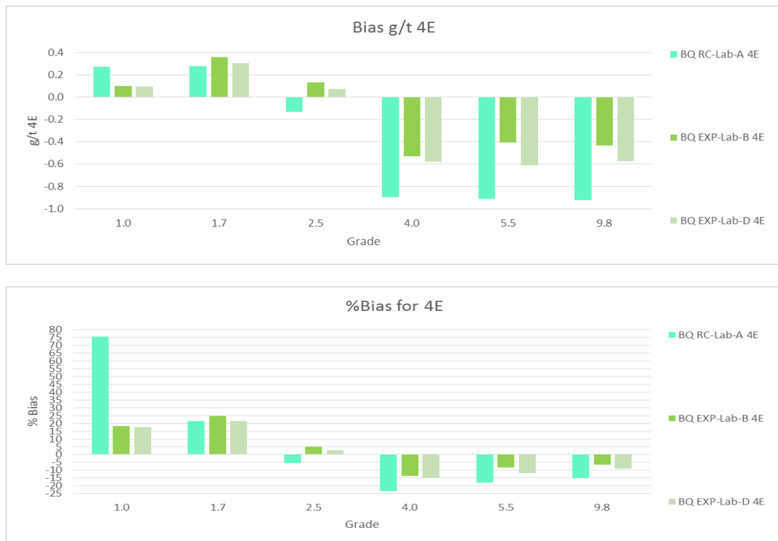
Figure 7-25 Analytical systematic errors GC-Lab vs. EXP-Lab quantified at the GCDPs for BQ sampling, in /t 4E and % Diff 4E
