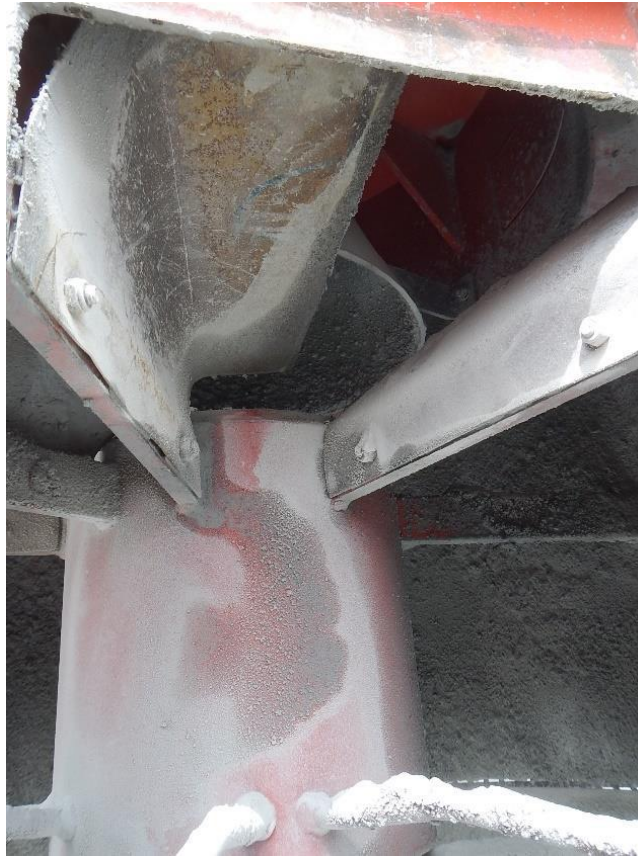
Figure 3-4 RC drill rig rota-port sampling cutter blades
