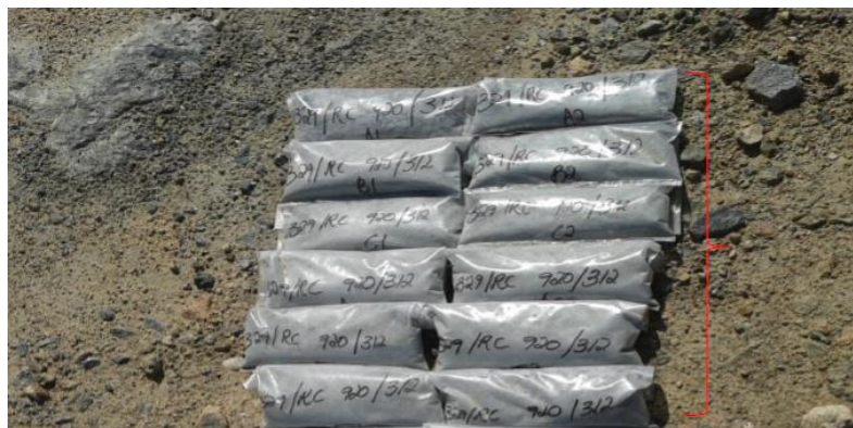
Figure 4-3 Reverse circulation samples prepared in the pit
