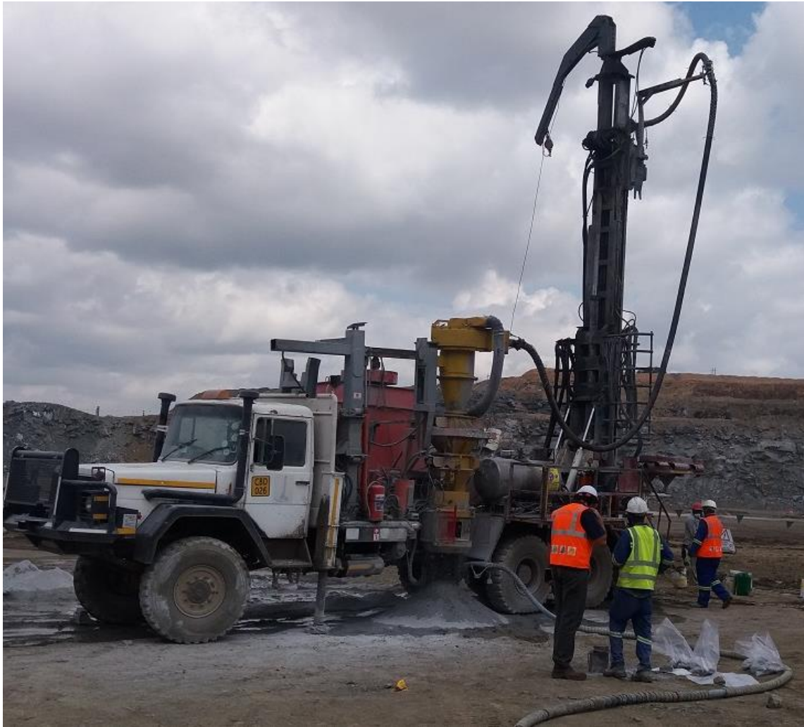
Figure 1-2 Reverse circulation drill rig used for grade control sampling at the platinum mine (13)
