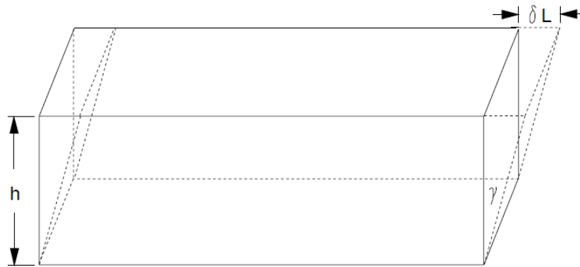
Figure 2-12 Shear deformation of a rectangular bar [53].
