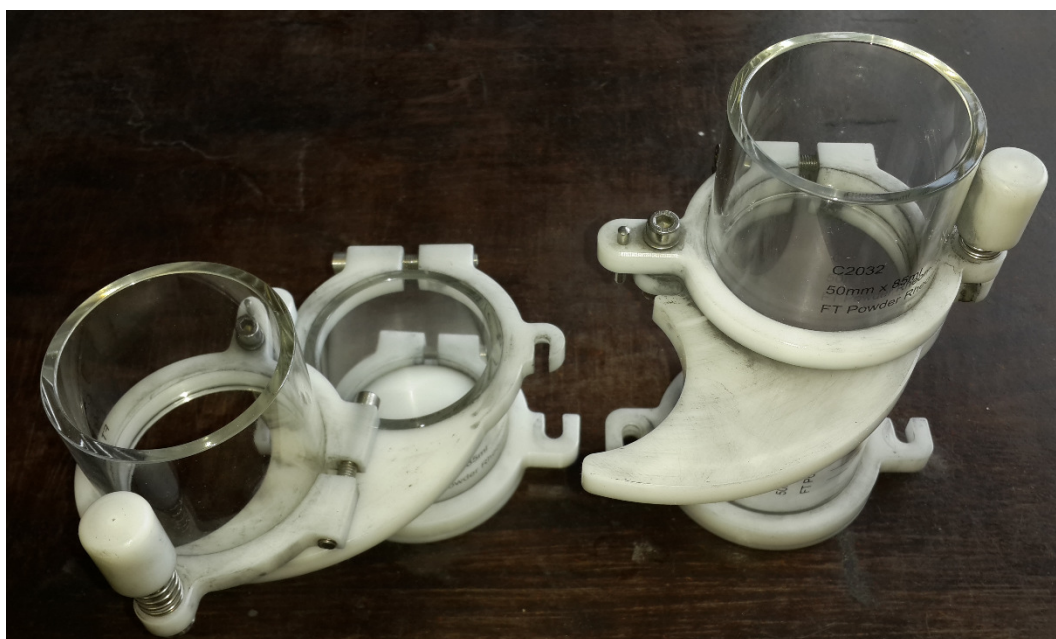
Figure 3-5 Split vessel assemblies used by the FT4 powder rheometer. Left: 85mL split vessel in the open position. Right: 160mL split vessel in the closed position.
