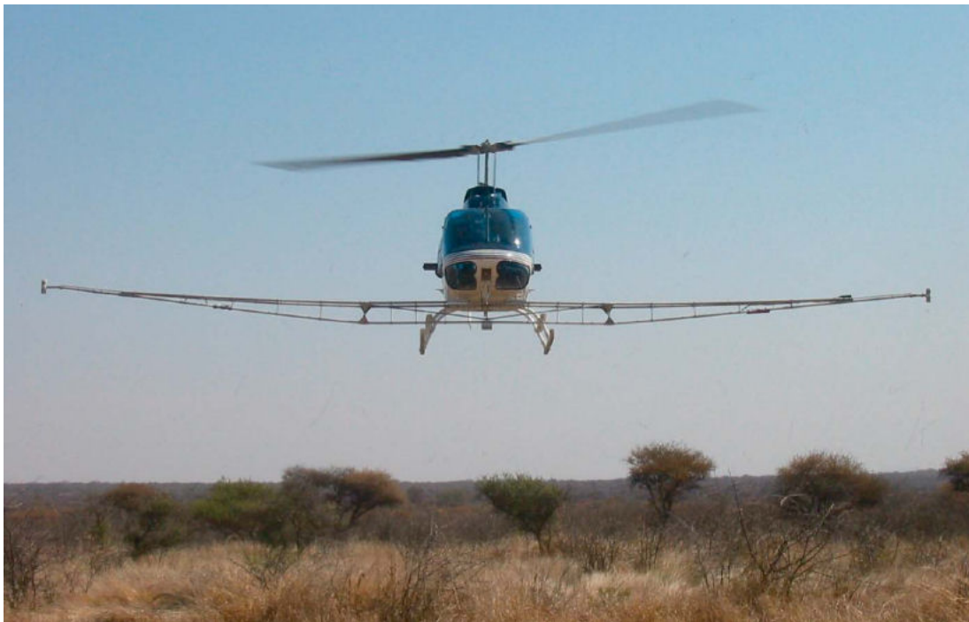
Figure 4.6 – JetRanger Bell 206 IIIB, with horizontally mounted magnetometers (Fugro, 2005).
