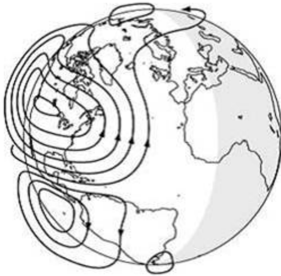
Figure 4.3 – Dynamos in the upper atmosphere generating magnetic fields which causes the diurnal (USGS, 2005).
