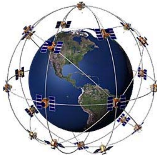
Figure 2.3 – Schematic diagram of the orbital paths of the 24-satellite constellation of the GPS system, orbiting the Earth at an altitude of approximately 20 200 km. Note: diagram not to scale (Garmin, 2007).
