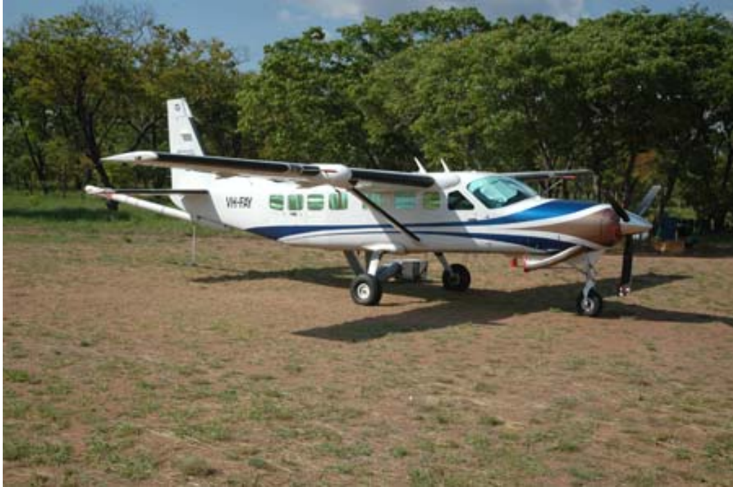
Figure 3.3 – Cessna Grand Caravan, modified to house the FALCON ® system for airborne surveys (BHP Billiton, 2007).
