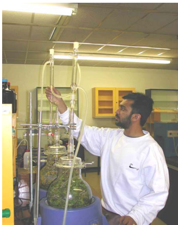
Figure 2: Plants being hydro-distilled using a Clevenger apparatus.
