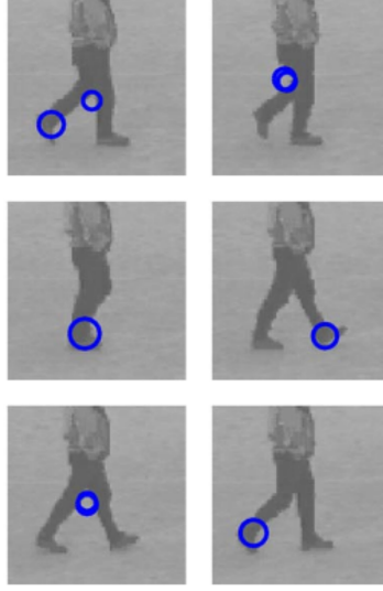
Figure 2.2: Example of detected STIP interest points [6]. These frames relate to the action walking from the KTH dataset. For the action of walking, intuitively, interest points would be things like joints such as ankles, knees, and similar areas. This is because they relate directly to the action of walking and walking can be defined by these areas and their associated motion. We can see that the STIP detector detects such points, but not necessarily in every frame. It is important to note that this is a case with a simple background with no other unrelated motion that could possibly confuse the detector into detecting false positives.
