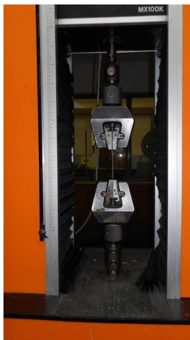
Figure 3.12. A photograph of a MX100K tensile testing machine that was used in this study.
