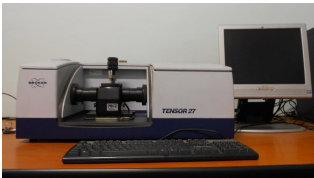
Figure 3.7. A photograph of a Bruker Tensor 27 Fourier transform infrared spectrometer that was used in this study.
