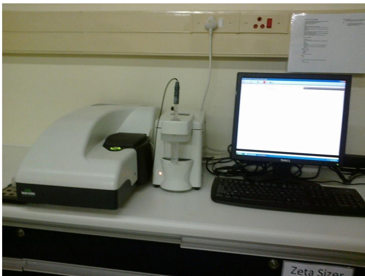
Figure 3.13. A photograph of a Malvern Zeta sizer machine that was used in this study.
