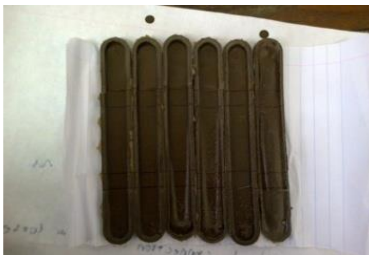
Figure 4.47. A photograph of a typical group of six specimens shown before being analysed for their tensile strengths.
