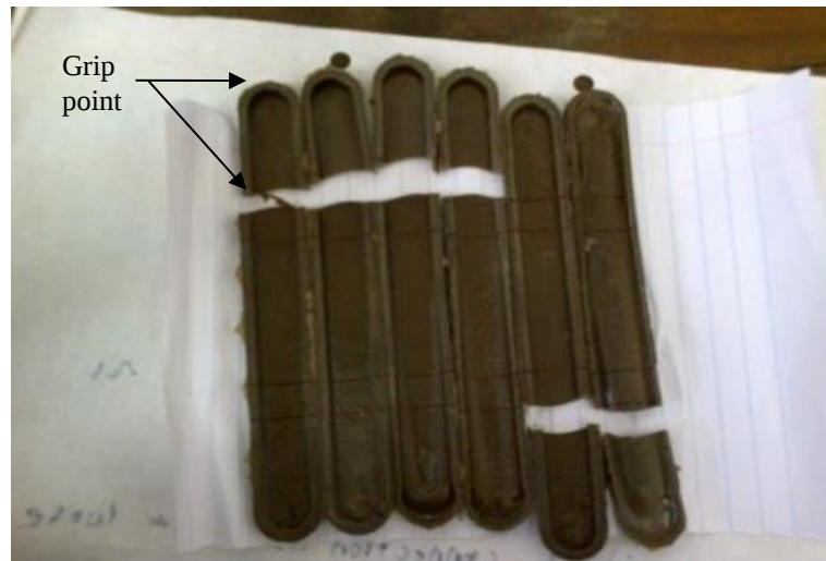
Figure 4.48. A photograph of a typical group of six specimens shown after being analysed for their tensile strengths. Notice the consistency of their break points.
