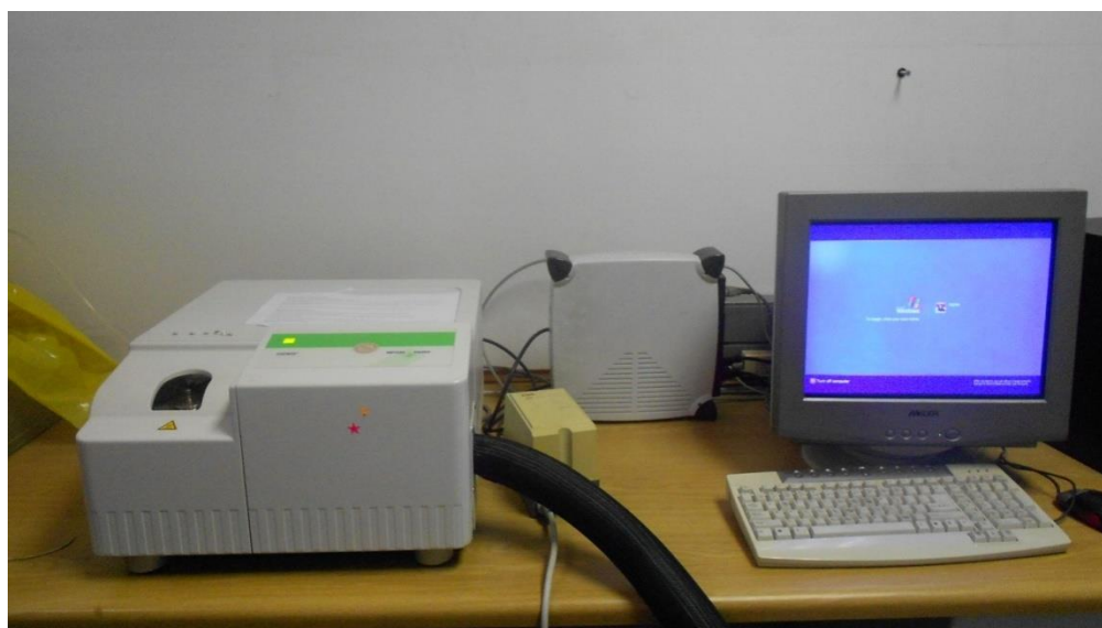
Figure 3.10. A photograph of a Mettler Toledo DSC 822e analyzer which was used in this study.
