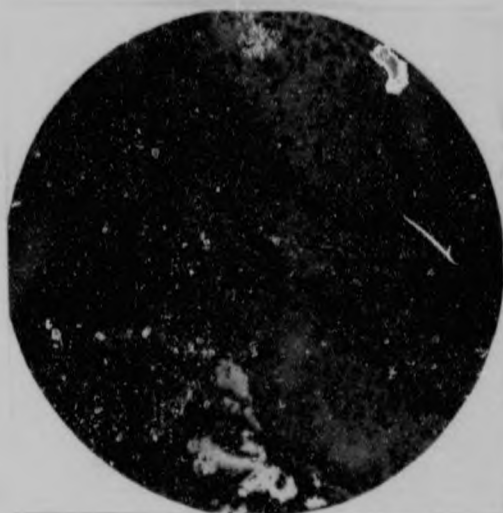
B. Tetrahedrite Veining Sphalerite.
