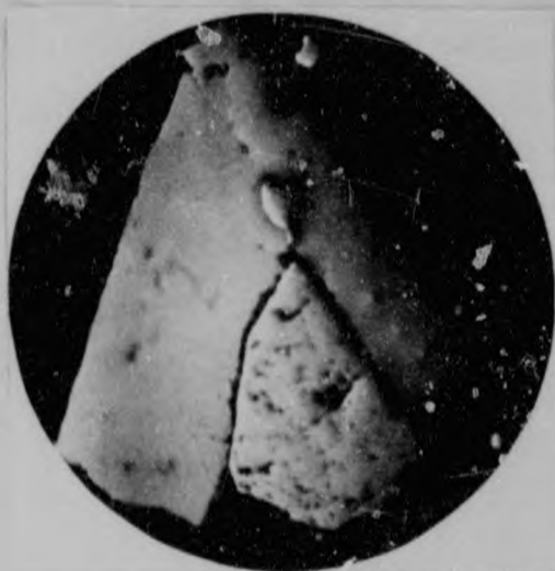
B. Twinned Arsenopyrite Crystals Replacing Pyrite.
