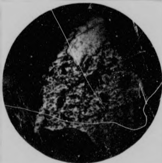
C. Gold associated with Coarser Pyrite.
