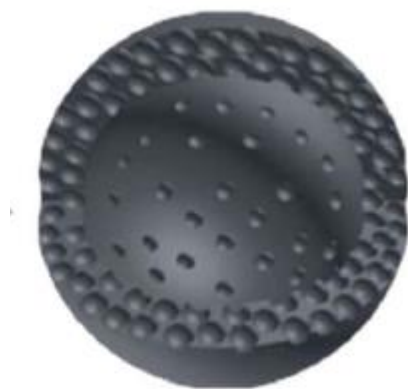
Figure 4.1 Structure of a hollow carbon sphere with a porous shell. 7
