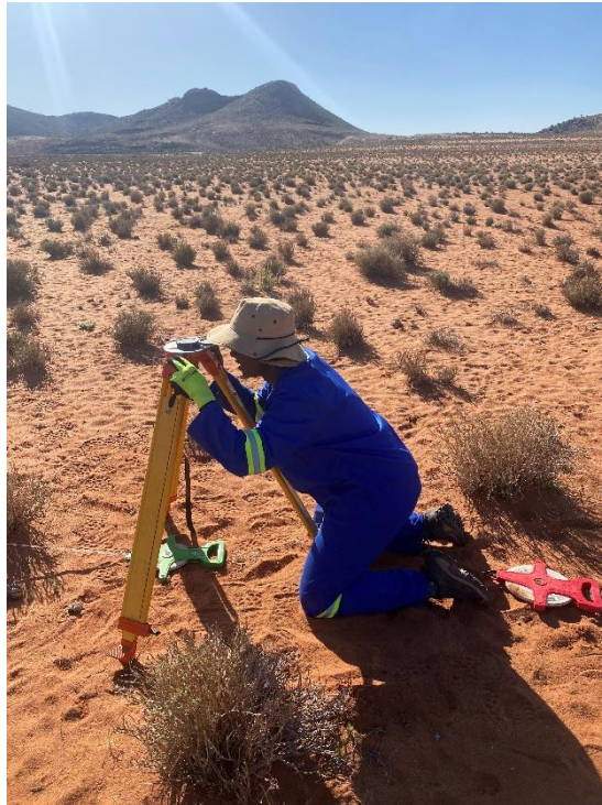
Figure 22: Image showing a geophysicist using a compass and tripod to locate the north, south, east, and west direction.
