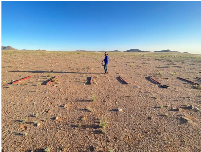
Figure 21: Image showing the magnetic induction coils being prepared for calibration.
