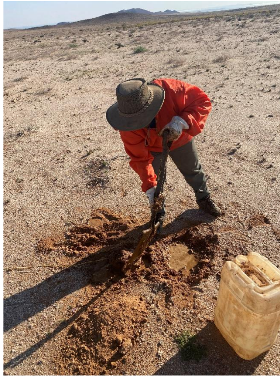
Figure 24: Image showing an electrode being buried in a salty water mud solution.
