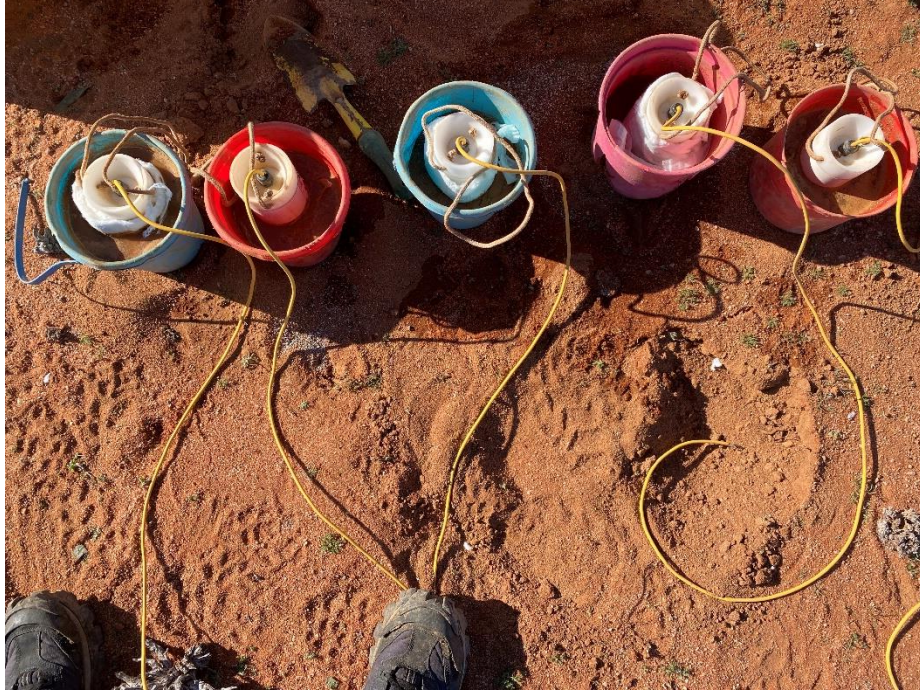
Figure 23: Image showing electrodes being placed inside a salt water and cat litter mud solution while covered with diapers for moisture retention.
