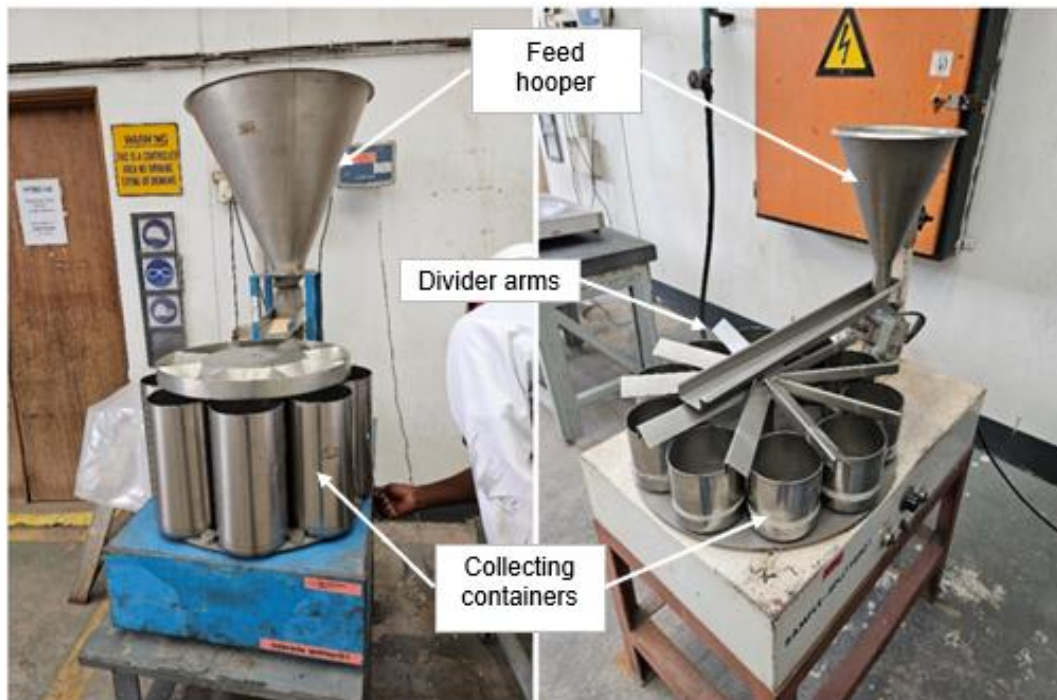
Figure 3.1. Rotary samplers that were used to extract representative samples from the bulk.
