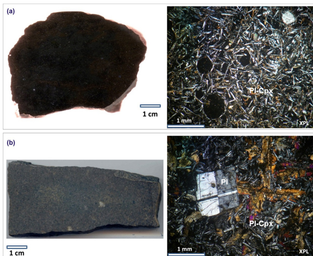
Figure 6.4. Dolerite samples. (a) RPS056 from the SJ Dome showing spherulitic textures (right). Spherulites are generally microcrystalline to cryptocrystalline intergrowths of quartz, calcite and other phases. (b) RSS048 sampled from a series of dolerite dykes that intrude the hinge zone of the Blauer Heinrich syncline, in this case from the lower section of the Khan Mine Gorge where it can be seen to be a plagioclase-phyric ilmenite-bearing dolerite. PPL – plain polarised light, XPL – cross polarised light. For an explanation of mineral abbreviations refer to Appendix I.
