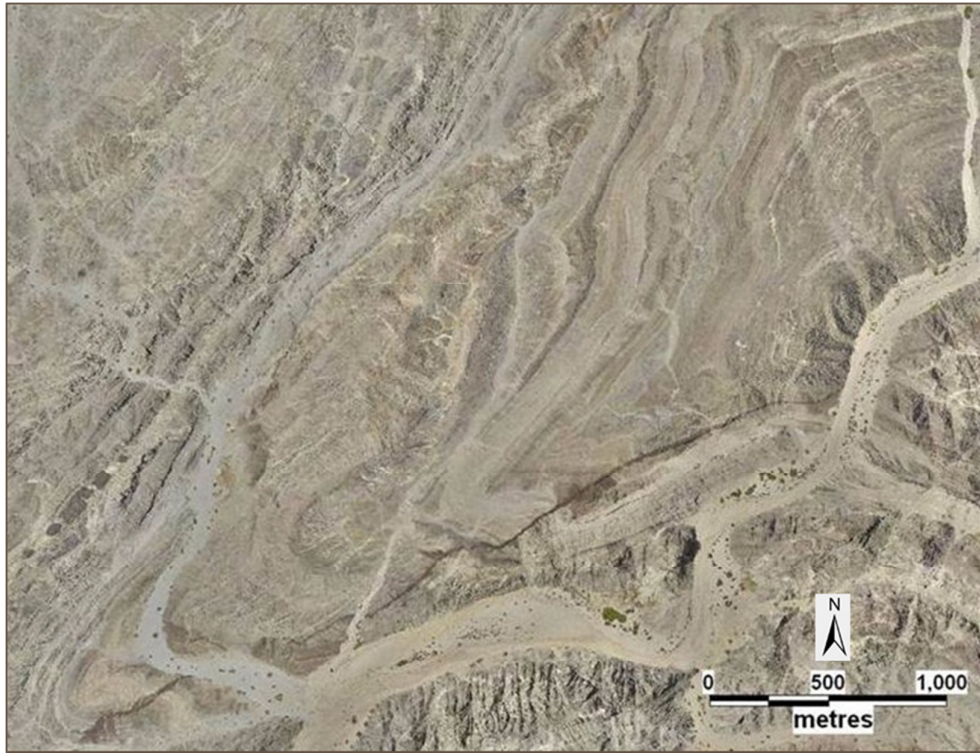
Figure 2.15. Example of a portion of the ortho-rectified aerial photographic mosaic surveyed and produced by Southern Mapping Company for Rössing Uranium Ltd. in 2008. The image has a 15 cm spatial resolution and covers the Blauer Heinrich Syncline area along the Khan River. A dolerite dyke cuts the hinge zone parallel to the fold axial plane. Note trees in the river bed for scale. Figure is centred on 501000 mE, 7508000 mN. The location of the Blauer Heinrich Syncline is shown in Figure 4.1.
