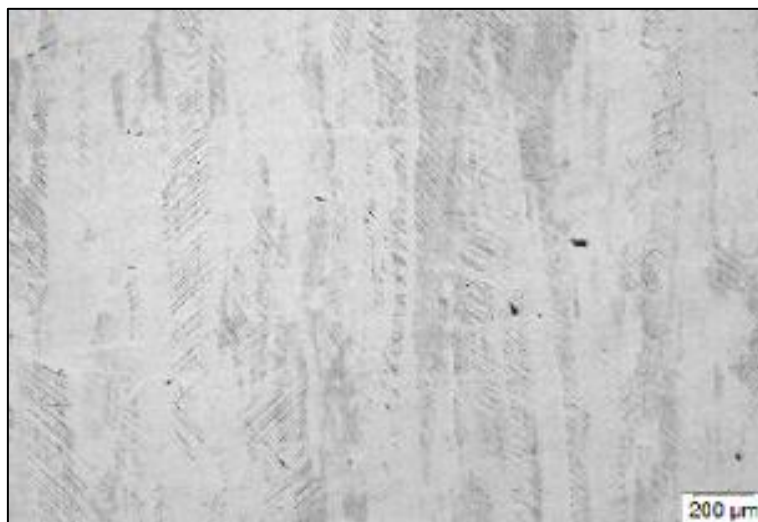
Figure 2-7 - The microstructure of Ti-6Al-4V produced by L-PBF [13].
