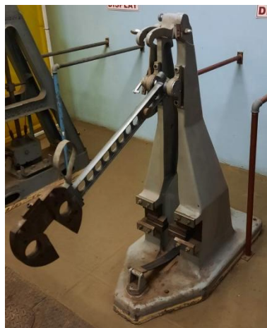
Figure 4-3 - The Charpy impact tester of the material labs at Wits.
