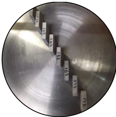
Figure 5-3 - Manufactured blocks on the baseplate for the final experiment.
