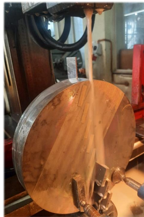
Figure 5-4 - EDM wire cutting of printed blocks from the base plate.
