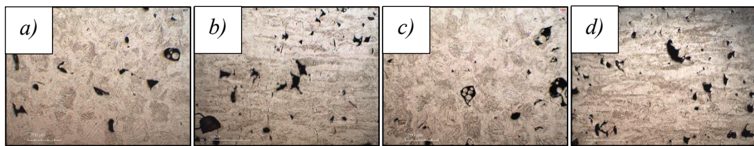
Optical Microscope images of etched 142 \mu\text{m} hatch samples in xy plane and yz planes: (a),(b) - microstructure of SR sample, (c),(d), microstructure of SR+LSP sample.
