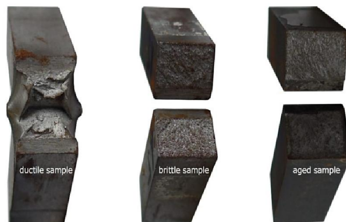
Figure 2-24 - Appearance of fractures in different types of Charpy samples [101].
