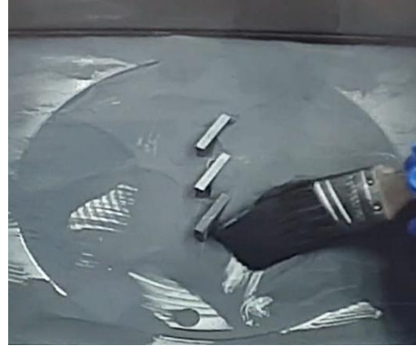
Figure 5-2 - Powder removal from the build chamber.
