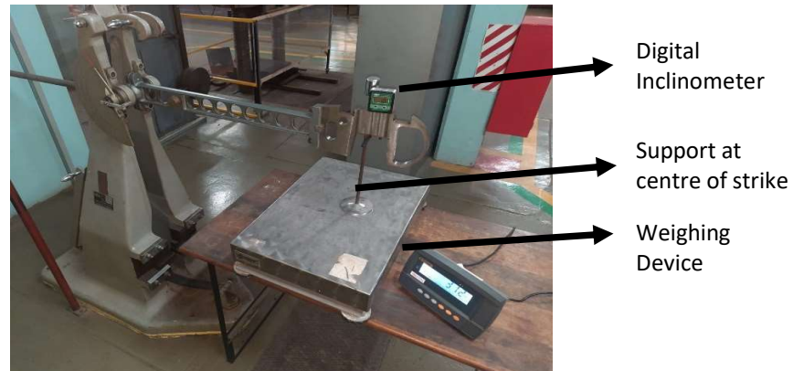
Figure 3 pendulum arm set horizontally to measure the supporting force
