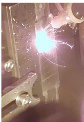
Figure 5-10 - LSP of MCVN samples held in jig.
