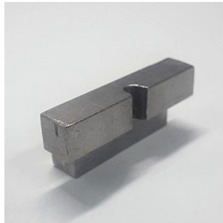
Figure 4-5 - Centring jig designed for the new anvils.
