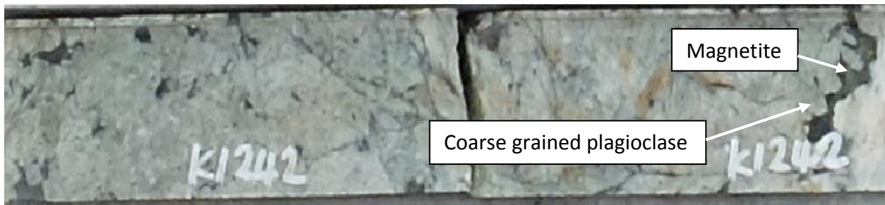
Figure 4.9: Anorthosite of the lower lithologic unit of HW029 at a depth of 592.4. Note the interstitial magnetite and coarse-grained plagioclase grains.
