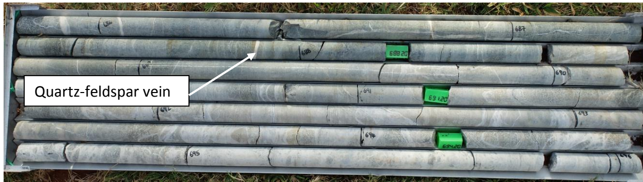
Figure 4.10: Calcsilicate xenolith of the lower lithologic unit from HW029 at depth of 686-696 m. Note quartz-feldspar veins.
