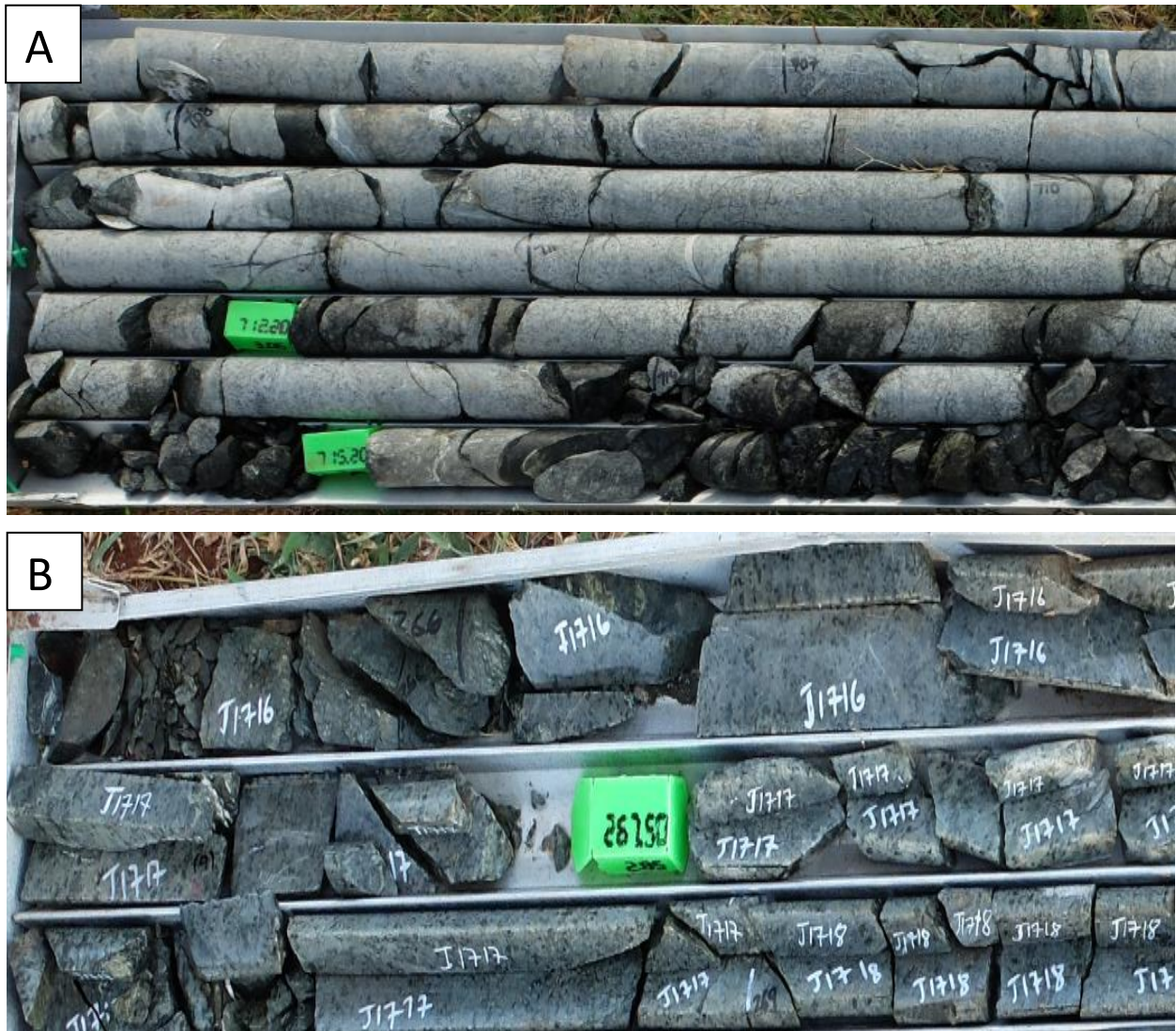
Figure 4.8: Gabbros of the lower lithologic unit. A) Gabbro from HW029 at a depth of 709.2-716 m. B) Leucogabbro from HW029 at a depth of approximately 265-271 m.
