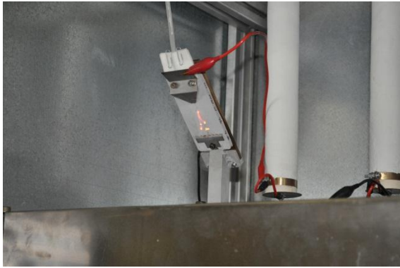
Figure C.38: “Long” scintillations observed
