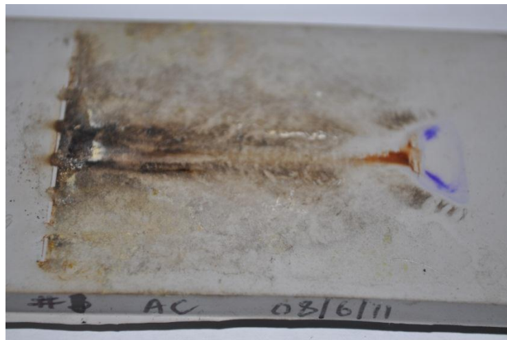
Figure C.14: Erosion and arc spots at ground end
