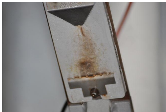
Figure C.19: Discolouration along length
