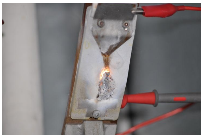
Figure C.24: Length of erosion on sample 3 progressed to 60%
