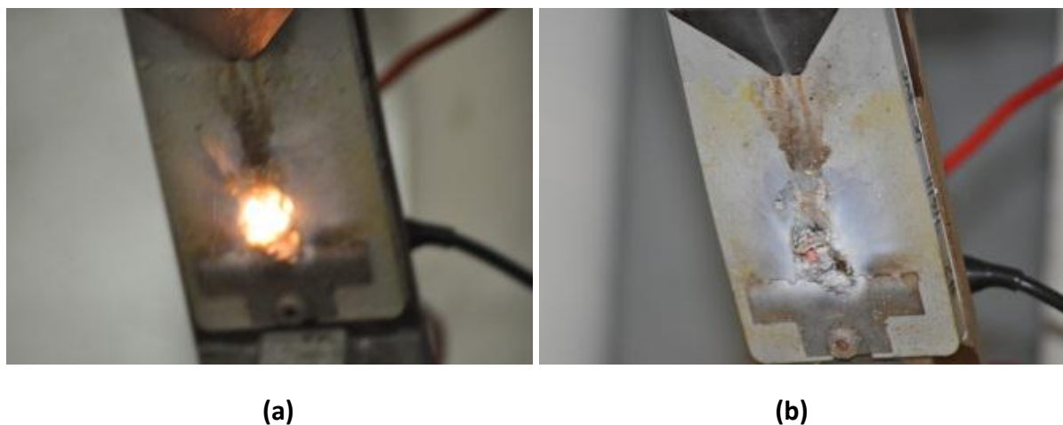
Figure 8: (a) Burning on sample 2 at ground electrode and; (b) erosion noted on sample 2
