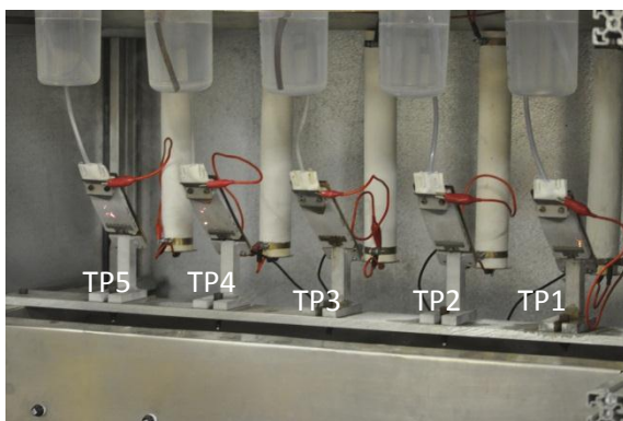
Figure C.2: Discharge activity at start
