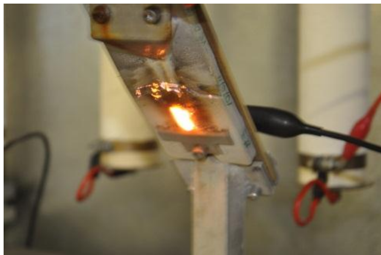
Figure 16: Development of arc roots with scintillations across the sample surface
