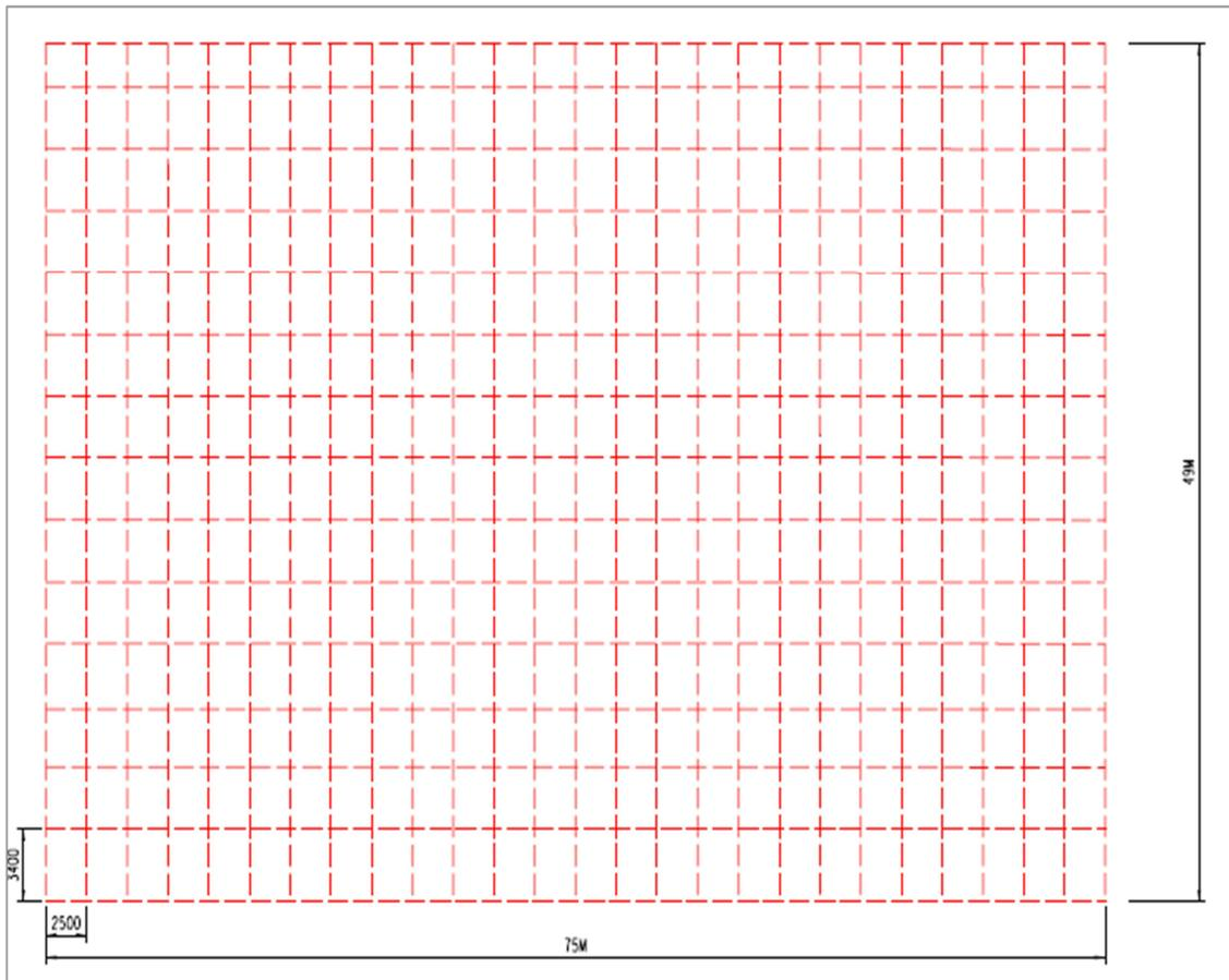
Figure 5. An Improved Ruighoek substation earth mat configuration
