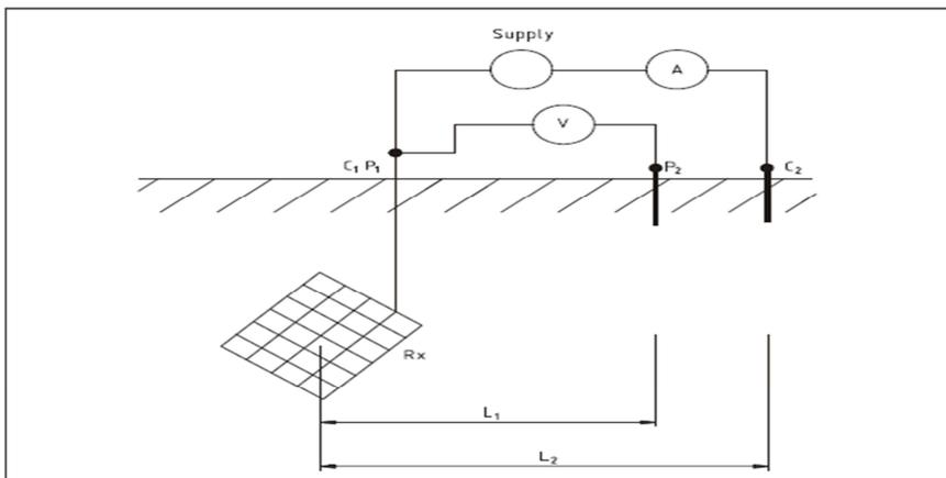
Figure 2: Fall of potential method for measuring earth resistance [7, 13].
