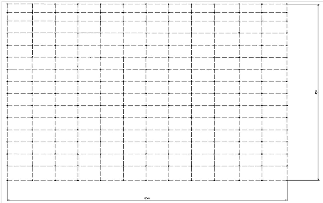
Figure 4: Existing Ruighoek substation earth mat configuration [2].
