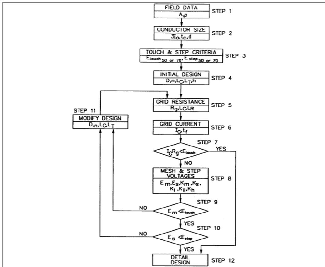
Figure 3: Design procedure block diagram [7].
