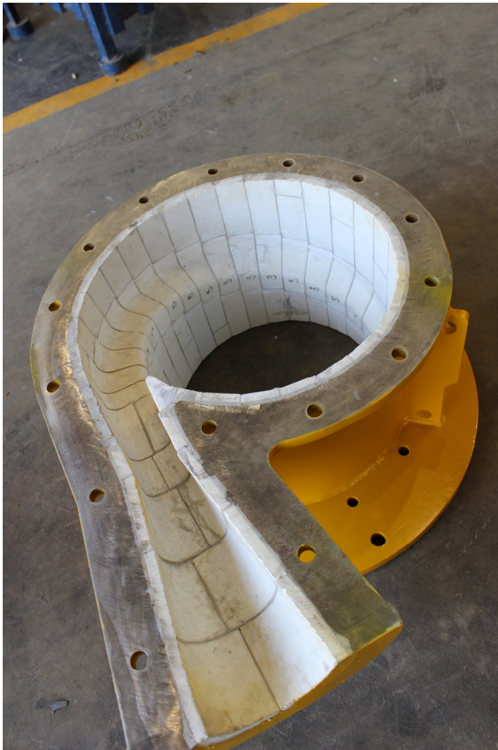
Figure 4.1.1. Cavex inlet geometry – tiled (CVXT)
