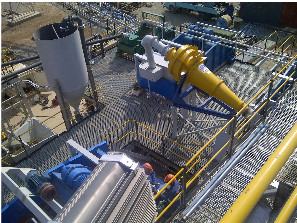
Figure 4.2.1. 650CVXT installed at a Fluorspar DMS plant
