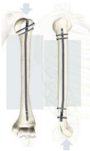
Figure 1.5. Antegrade and retrograde nailing techniques of the humerus. 24
