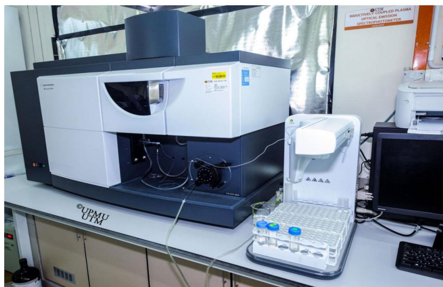
Figure 3-11: ICP-OES to analyse the samples.
