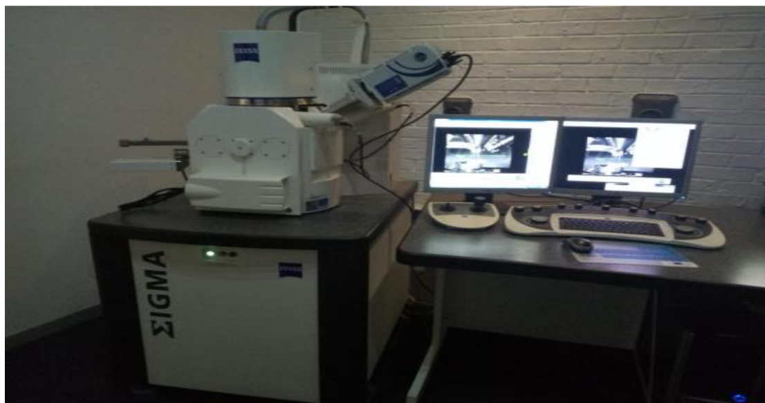
Figure 3-7: Carl Sigma Field Emission Scanning Electron Microscope equipped with an Oxford X-act EDS detector
