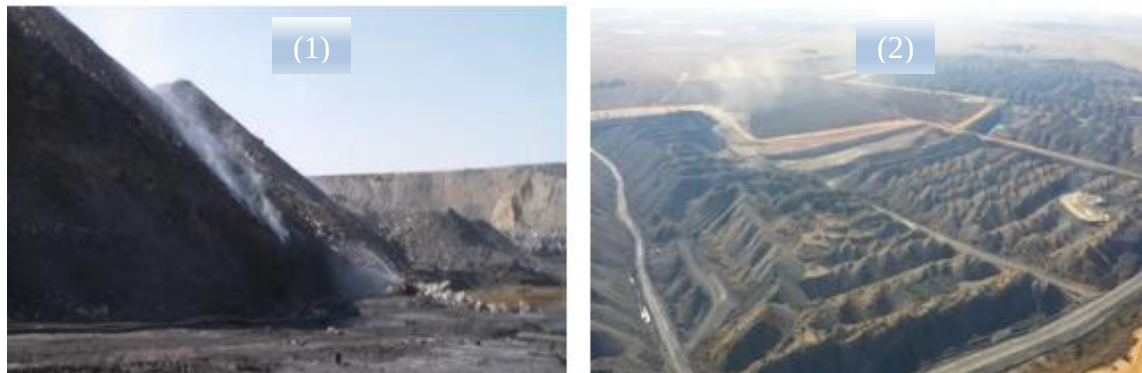
Figure 2-4: (1) Self-heating of run -of-mine fines, (2) Aerial view of Mpumalanga Highveld coal discard stockpile in South Africa (Rights, 2015)
