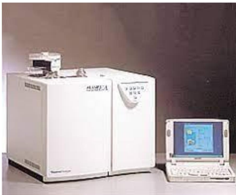
Figure 3-12 :Thermo Scientific Flash EA 1112 Elemental Analyser
