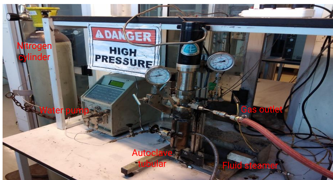
Figure 3-3: Image of hydrothermal experiment set up
