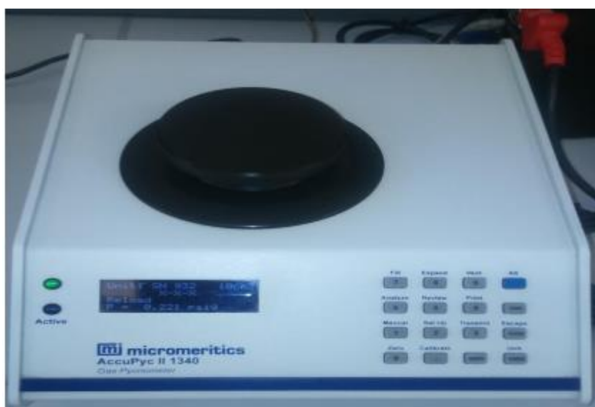
Figure 3-5: Micromeritics Accupyc II 1340 Pycnometer
