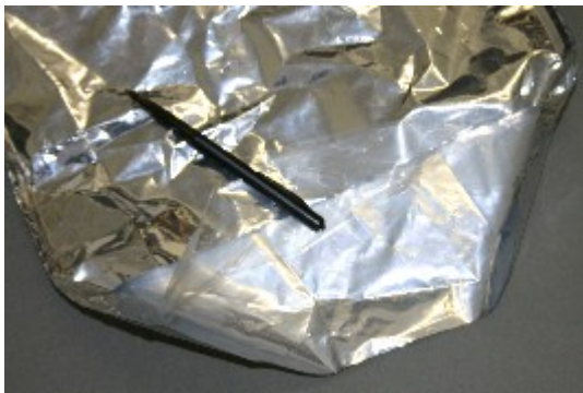
Figure 8: Wine bag cut open to show the laminate
