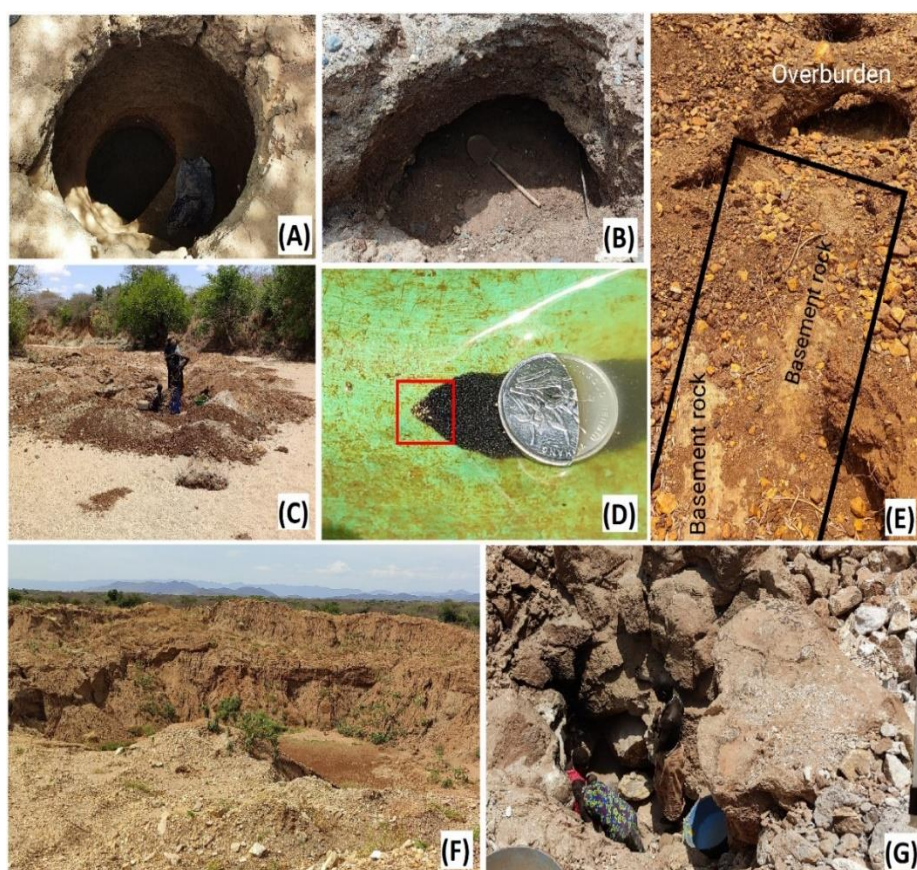
Figure 5.24: Field photographs showing workings /activity of the artisanal mining of alluvial gold deposits (A) Artisanal mining pit at Kaitap (B) site where overburden has been removed for panning (C) Two Toposa girls panning gold at Buno stream bed (D) shows gold nuggets in the red square recovered from alluvial sediment from Buno stream (E) overburden and basement rocks (F) Open pit where the overburden is recovered using an excavator pan with the Didinga Hills on the horizon (G) Three Toposa girls in Kawokono recovering sediments deposited between marble boulders to be panned for gold.
