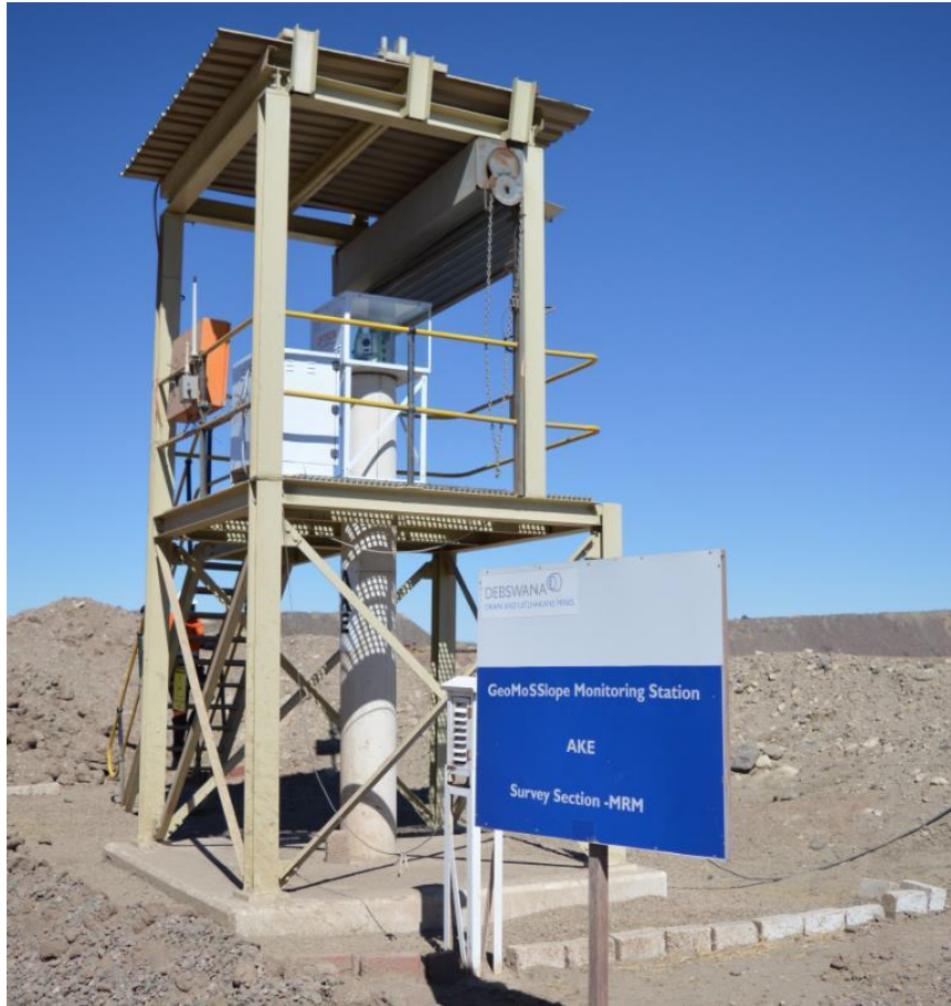
Figure 4.4: Leica GeoMoS transfer beacon. Source: Orapa Survey Department.
