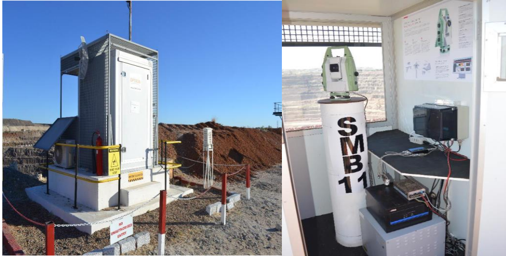
Figure 5.9: Shelter for transfer beacon. Source: Orapa Survey Department.
