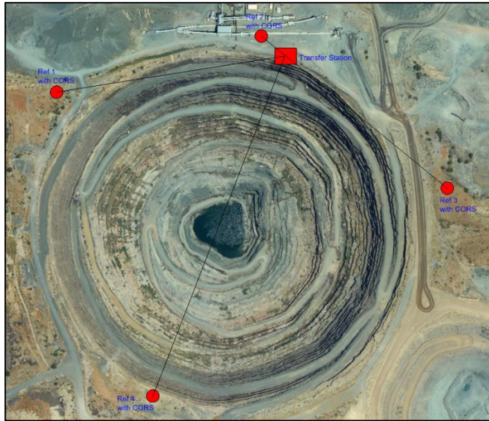
Figure 1.6: Layout of the CORS system. Source: Orapa Survey Department.
