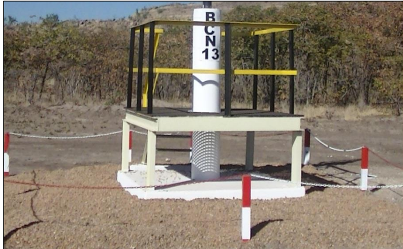
Figure 2.11: Reference beacon. Source: Orapa Survey Department
