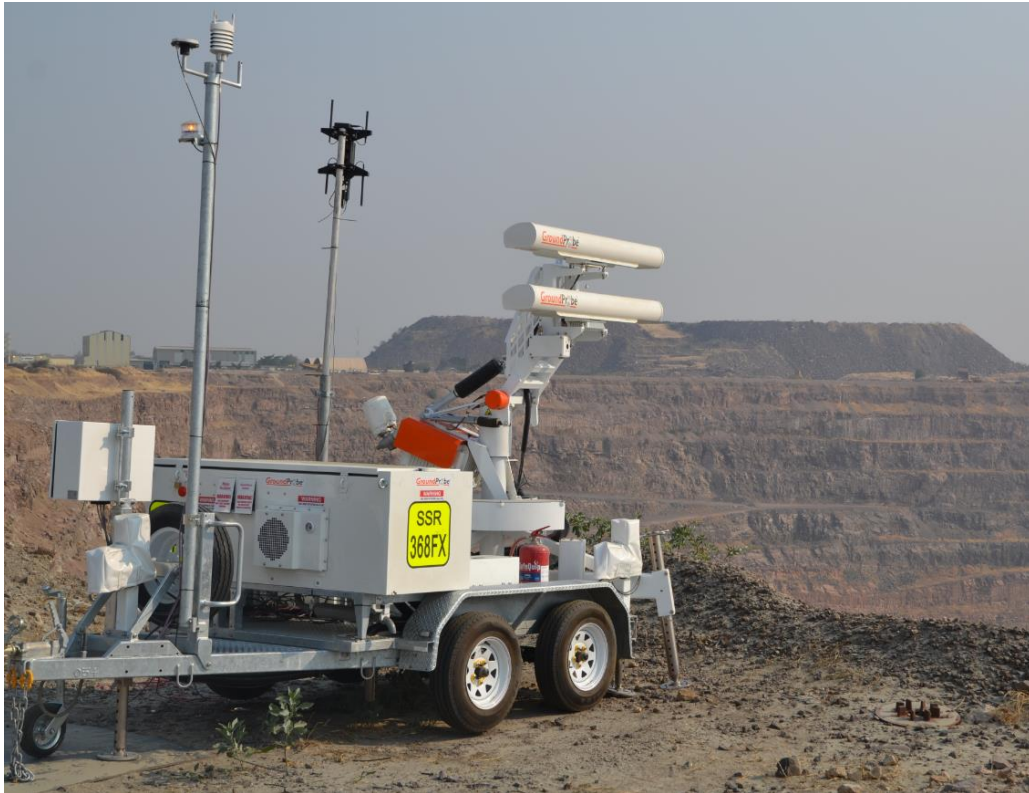
Figure 2.4: Using Radar to monitor a slope face. Source: Orapa Geotechnical Engineering Department.
