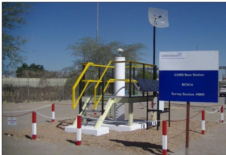
Figure 2.5: GNSS monitoring setup. Source: Orapa Survey Department.
