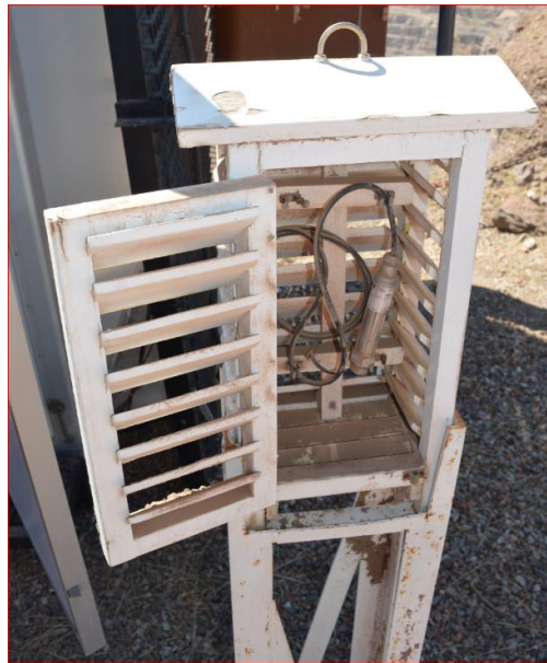
Figure 3.10: Meteorological sensor in a Stevenson Screen. Source: Orapa Survey Department.
