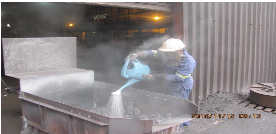
Figure 9: Equipment for the preparation of the borate solution for quenching
