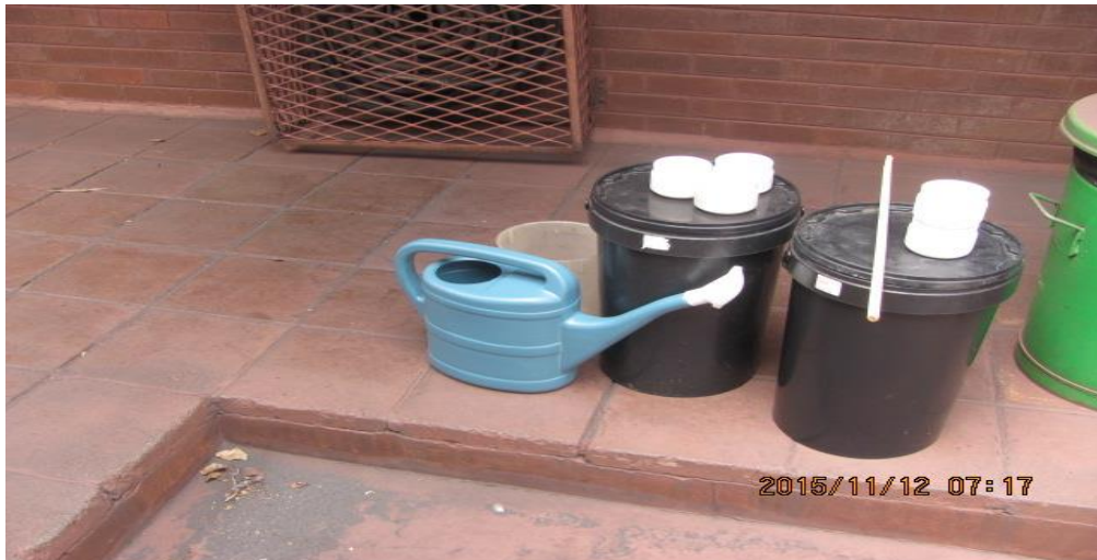
Figure 8: Equipment for the preparation of the borate solution for quenching
